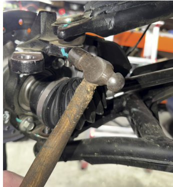
FIG 10 & FIG 11 - Remove knuckle and tie up out of the way
