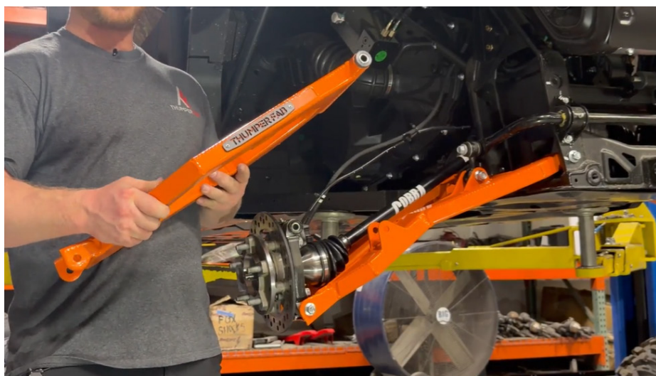
FIG 96 - Fasten the upper control arm to the frame
