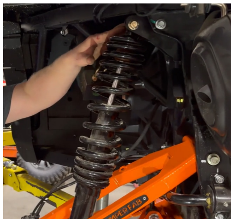
FIG 97 - Fasten rear shock to relocation brackets
