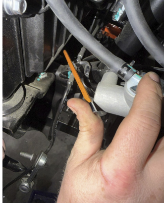
FIG 32 - Remove the OEM front brake lines
