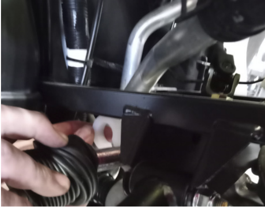
FIG 49 - Install Steering Stops
