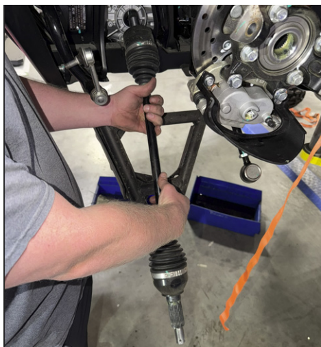
FIG 17 - Remove the front axles
