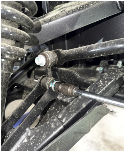
FIG 71 - Disconnect the rear sway bar from the lower control arm
