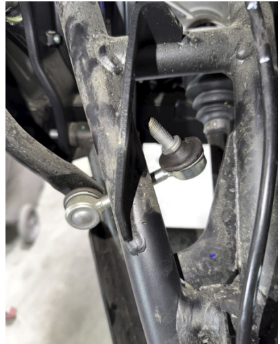
FIG 13 & FIG 14 - Disconnect sway bar from upper control arm
