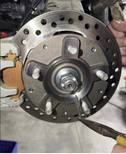
FIG 69 & FIG 70 - Remove the rear axle nuts
