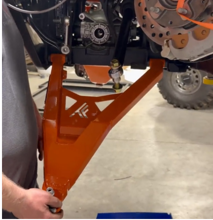
FIG 54 - Mount lower control arm
