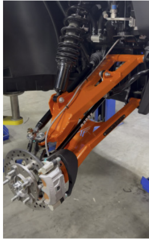
FIG 105 - Fasten front brake lines to control arms
