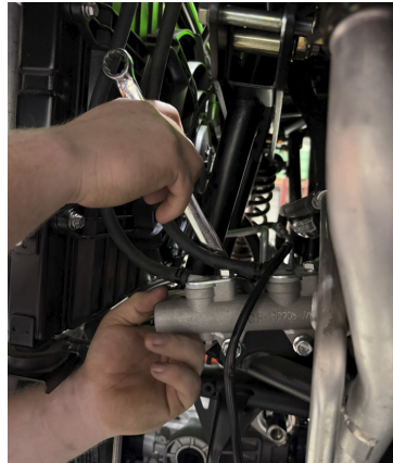
FIG 36 & FIG 37 - Fasten the new brake lines to master cylinder
