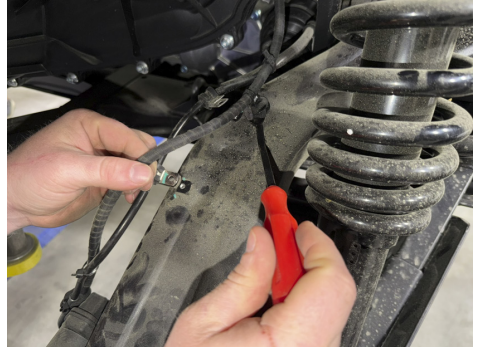
FIG 1 & FIG 2 - Drill out rivets that fasten the brake lines to the OEM control arms
