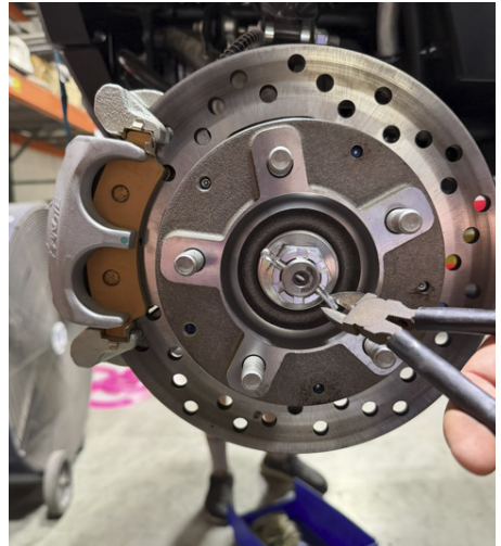
FIG 3 & FIG 4 - Remove axle nut cotter pins
