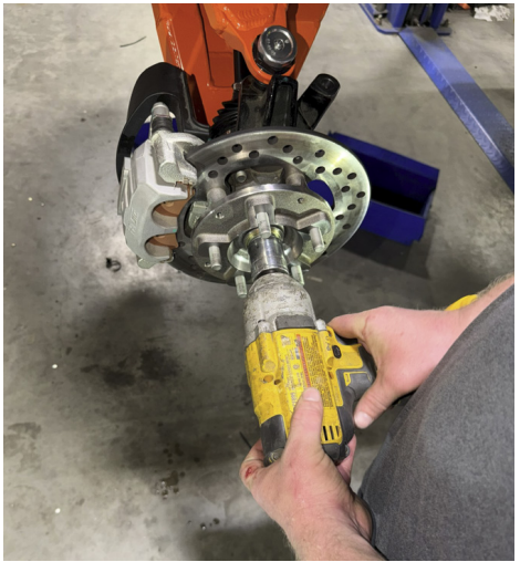
FIG 62 & FIG 63 - Install and tighten front axle nut
