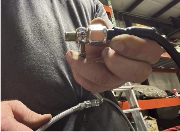
FIG 35 - Insert brake sensor through new master cylinder brake line
