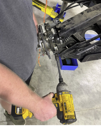
FIG 76 & FIG 77 - Remove the lower knuckle mounting bolt and tie the knuckle out of the way
