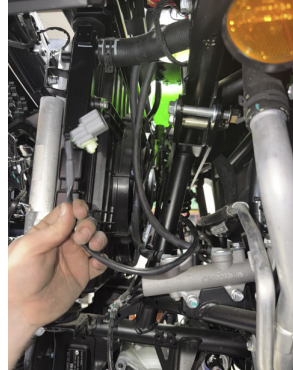
FIG 28 & FIG 29 - Remove brake fluid pressure sensor
