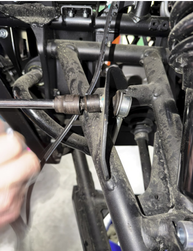
FIG 13 & FIG 14 - Disconnect sway bar from upper control arm
