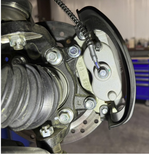
FIG 9 - Disconnect the front brake calipers
