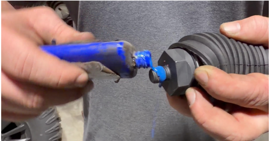
FIG 48 - Apply loctite to the inner tie rod
