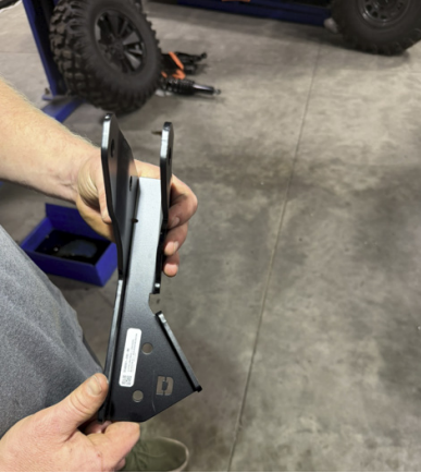
FIG 83 & FIG 84 - Insert the rear shock spacers into the rear shock relocation brackets
