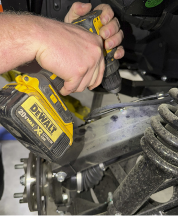
FIG 1 & FIG 2 - Drill out rivets that fasten the brake lines to the OEM control arms
