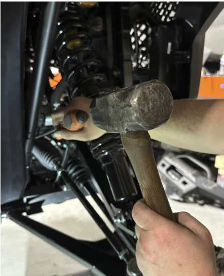
FIG 41 & FIG 42 - Remove OEM steering boot clamp
