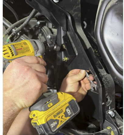
FIG 87 & FIG 88 - Fasten the Rear Shock Relocation Sandwich Plates to the frame and the Rear Shock Relocation Brackets
