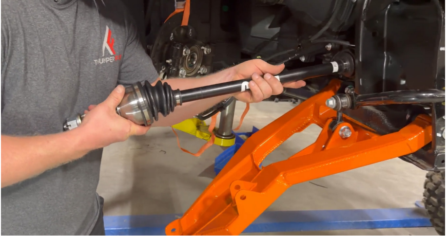
FIG 92 - Insert rear axles
