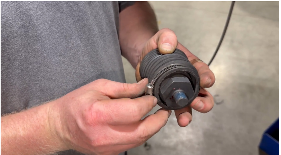
FIG 50 - Slide hose clamp over steering boot
