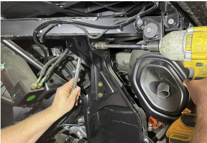
FIG 89 - Fully tighten the Rear Shock Relocation Bracket
