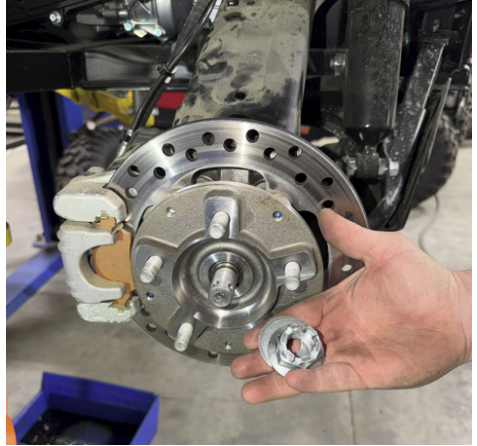
FIG 69 & FIG 70 - Remove the rear axle nuts
