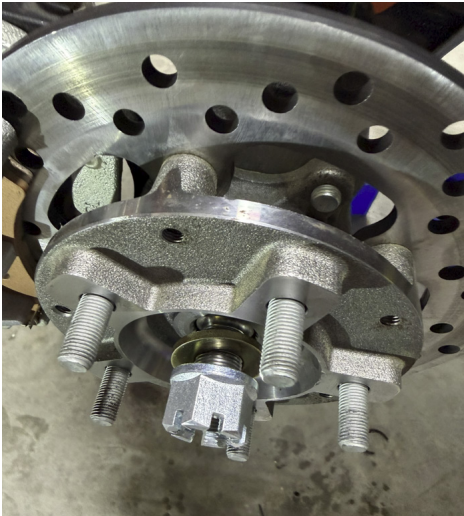
FIG 62 & FIG 63 - Install and tighten front axle nut
