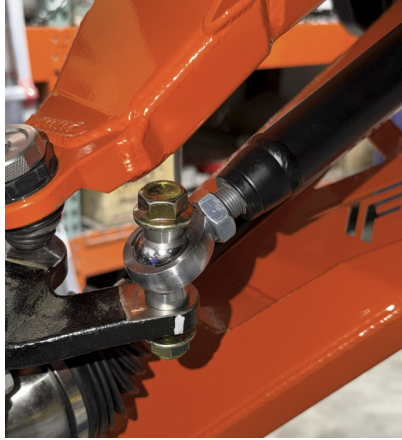
FIG 67 - Fasten the tie rod to the knuckle
