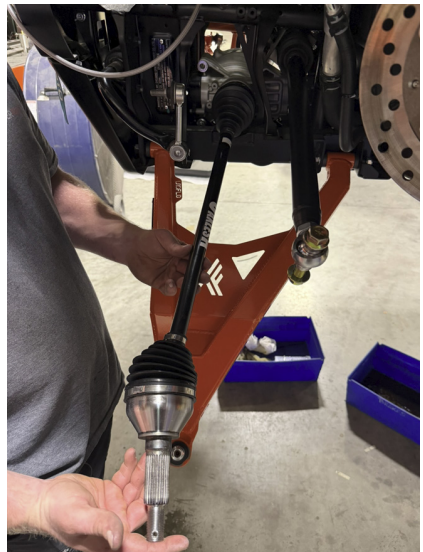
FIG 55 & FIG 56 - Install front axles
