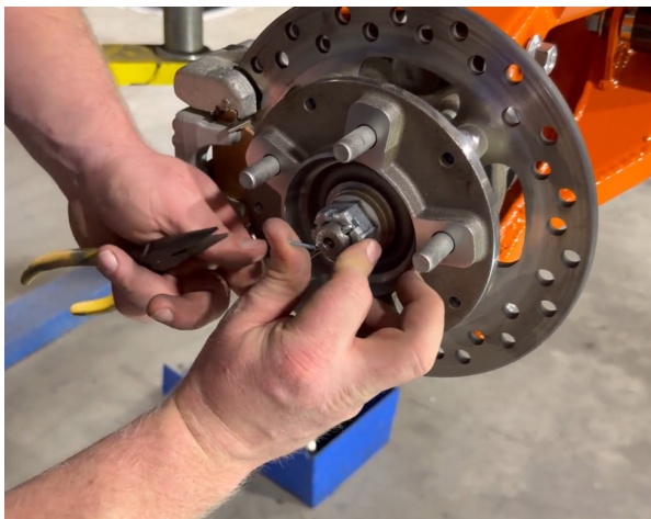
FIG 102 - Install cotter pin in rear axle nut
