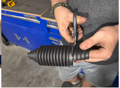
FIG 43 & FIG 44 - Trim the steering boot
