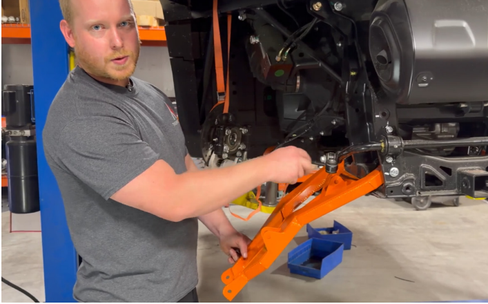
FIG 90 - Fasten the rear lower arm to the frame
