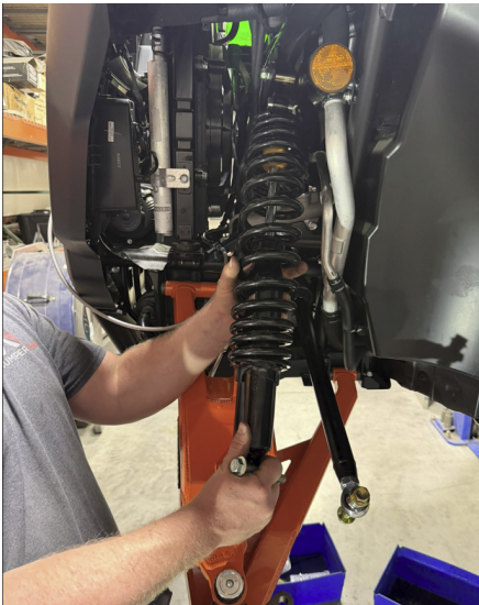
FIG 65 & FIG 66 - Install front shock
