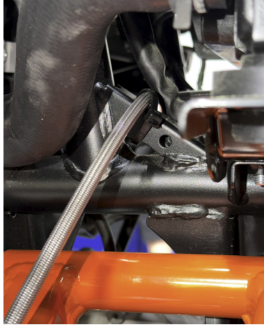
FIG 40 - Fasten the passenger brake line to the frame
