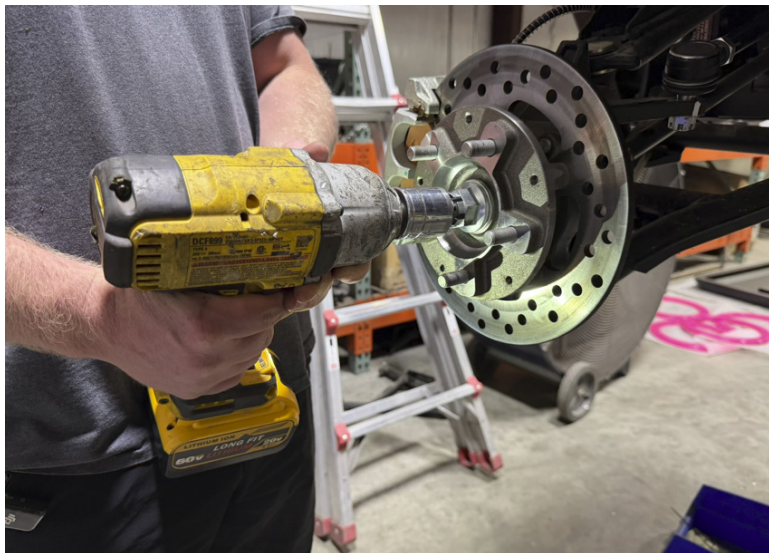
FIG 5 - Remove the axle nuts
