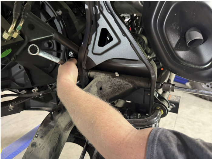
FIG 78 - Remove the upper control arm
