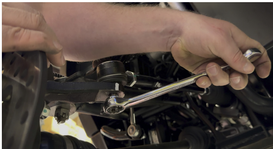
FIG 6 - Remove Tie Rod cotter pin and castle nut
