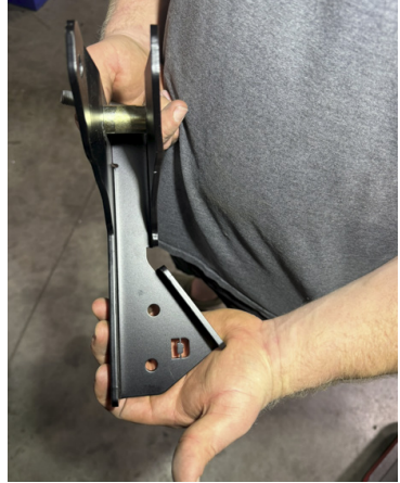
FIG 83 & FIG 84 - Insert the rear shock spacers into the rear shock relocation brackets
