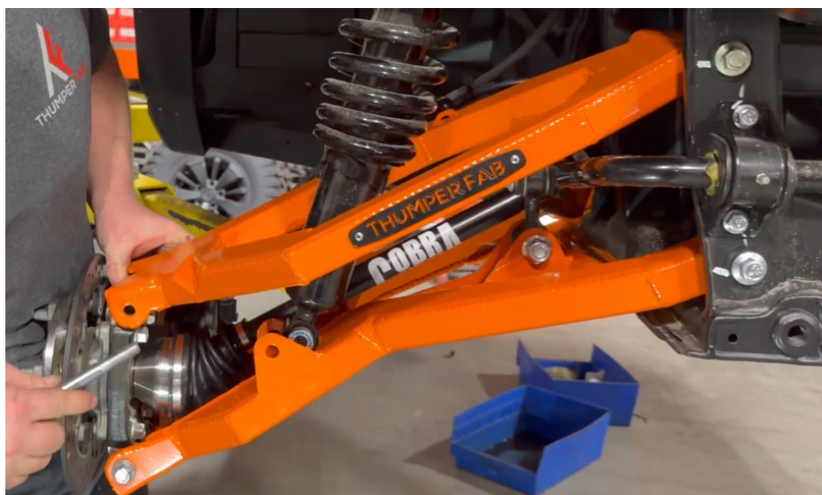
FIG 98 - Fasten the upper control arm to the knuckle
