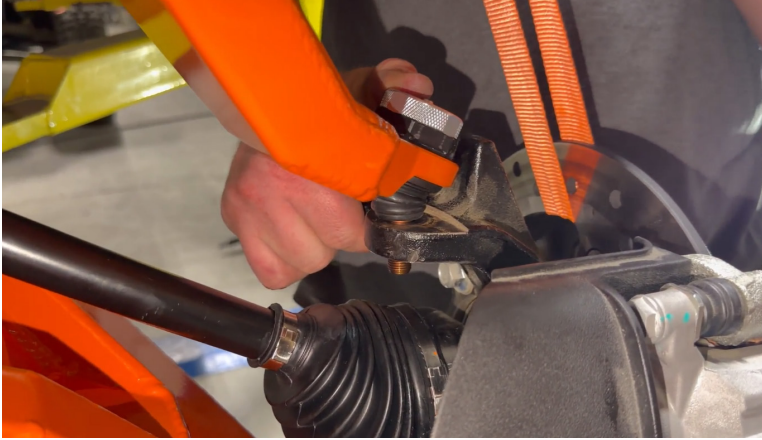
FIG 61 - Fasten the knuckle to the upper ball joint
