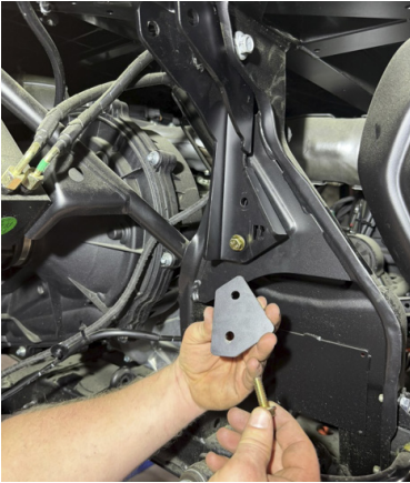
FIG 87 & FIG 88 - Fasten the Rear Shock Relocation Sandwich Plates to the frame and the Rear Shock Relocation Brackets
