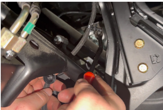
FIG 95 - Create extra brake line slack if needed
