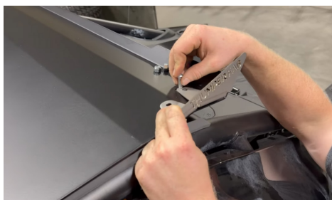
FIG 4 & FIG 5 - Loosley fasten rear of roof to roll cage
