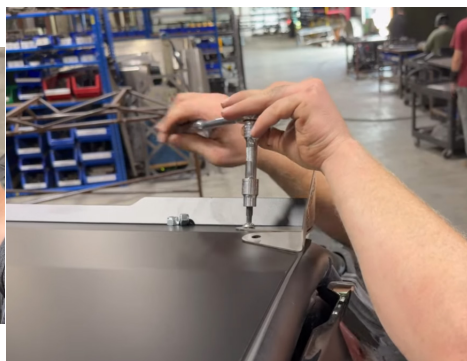
FIG 4 & FIG 5 - Loosley fasten rear of roof to roll cage
