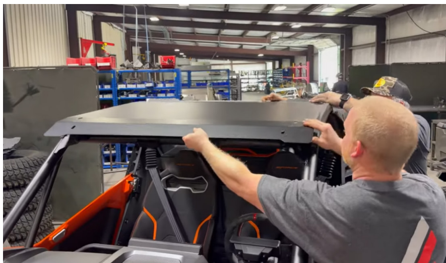
FIG 3 - Place the roof on top of the vehicle
