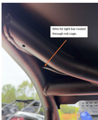
FIG 11 - Route the light bar wire through the roll cage
