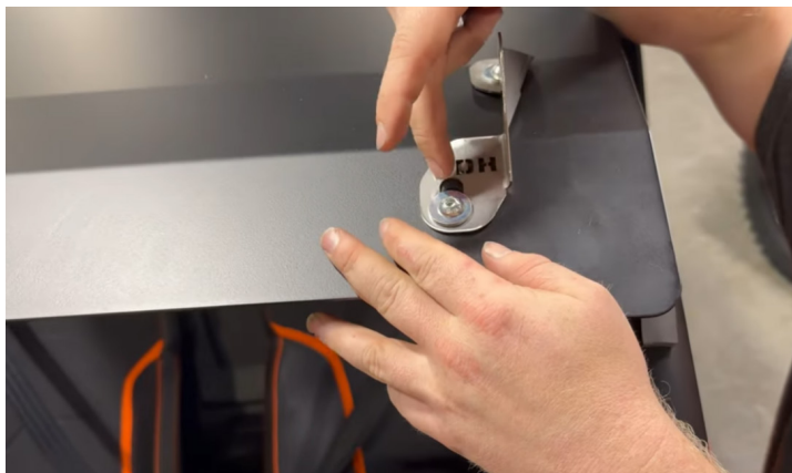
FIG 7 - Fasten the light bar brackets to the vehicle
