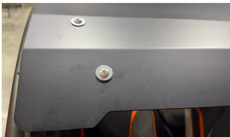
FIG 6 - Fasten the front of the roof to the roll cage
