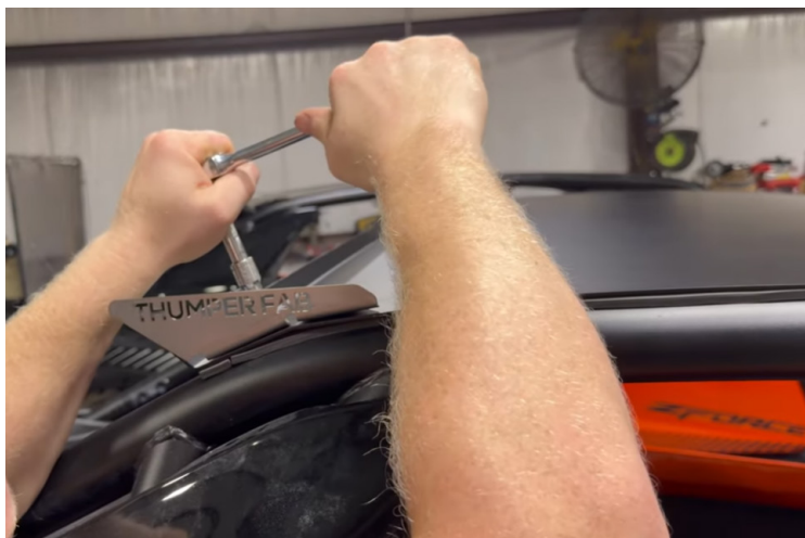
FIG 8 - Tighten remaining roof hardware
