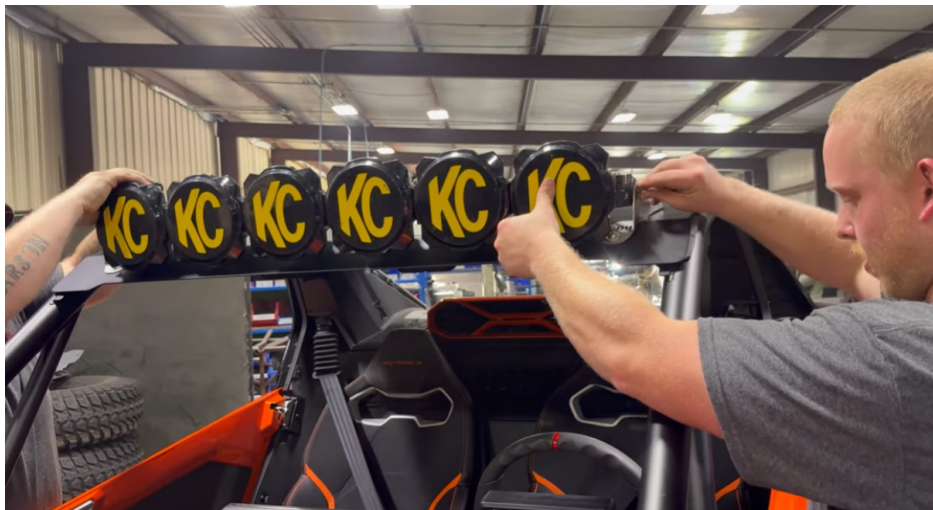
FIG 9 - (OPTIONAL) Fasten the light bar to the vehicle
