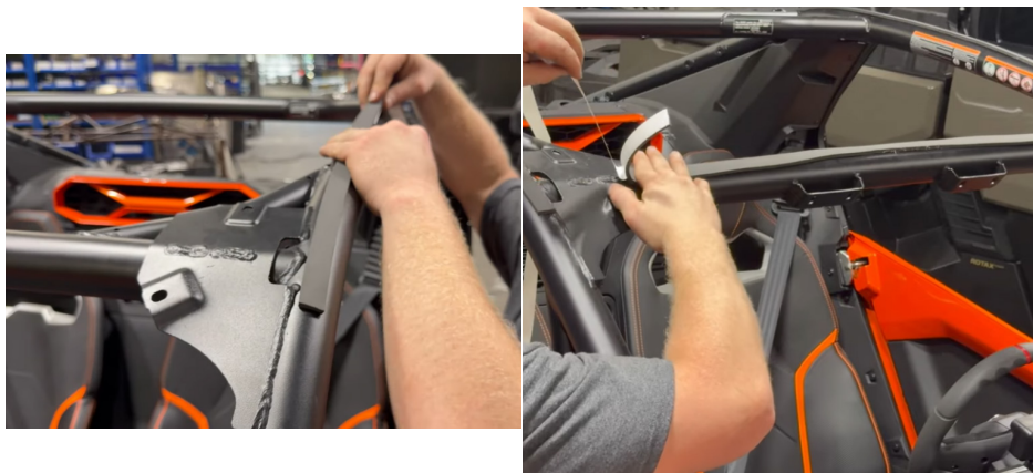
FIG 1 & FIG 2 - Apply foam to roll cage
