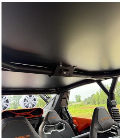
FIG 17 - Mount dome lights and dome light mount to underside of roof
