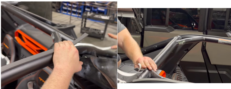
FIG 1 & FIG 2 - Apply foam to roll cage
