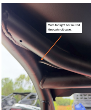
FIG 13 - Route the light bar wire through the roll cage
