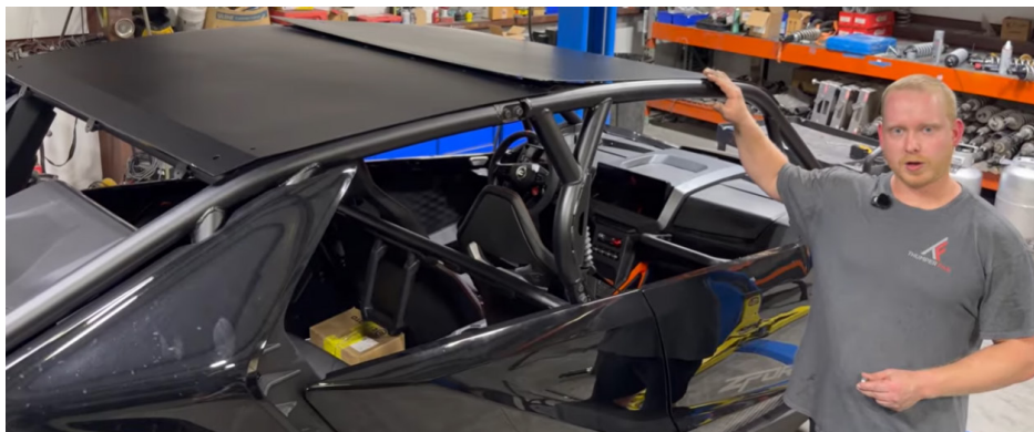
FIG 4 - Place the front of roof on the roll cage
