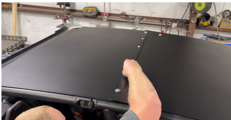
FIG 10 - Fasten the front and rear roof sections together
