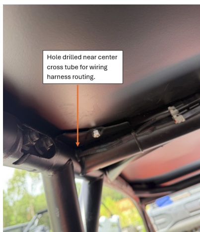
FIG 18 - Drill a hole in the roll cage near the center cross tube and route the harness up from the A-Pillar
