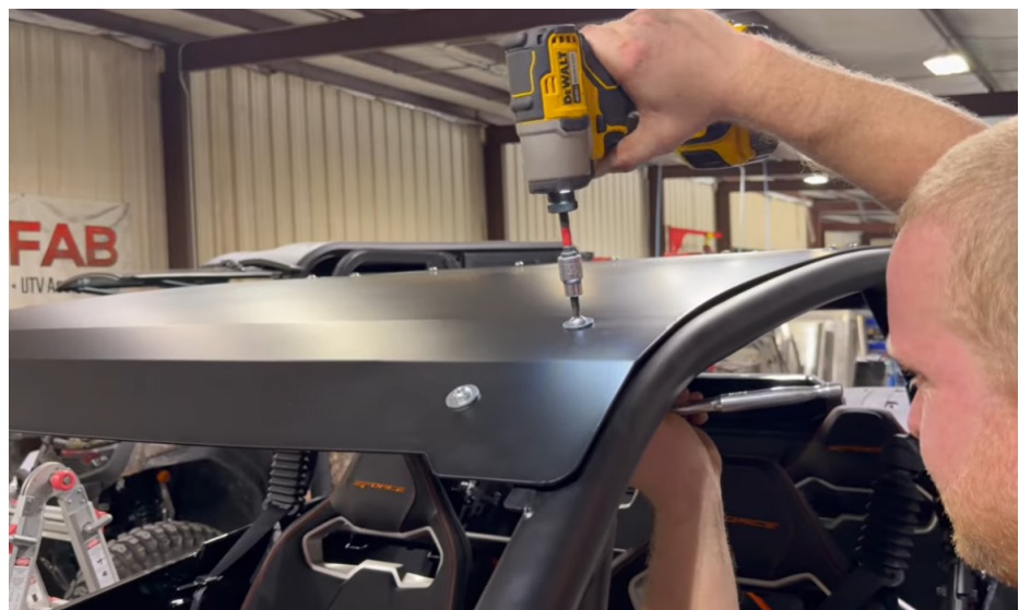
FIG 11 & FIG 12 - Tighten all Roof hardware
