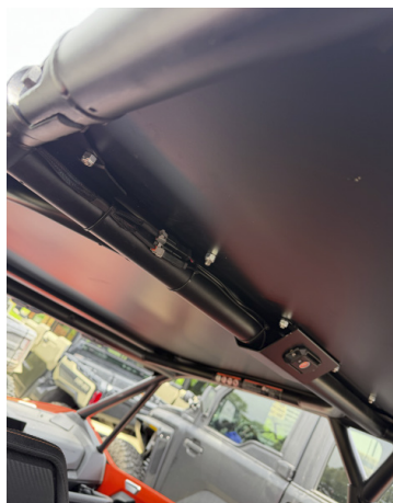
FIG 19 - Fasten wiring harness to center cross tube using zip ties
