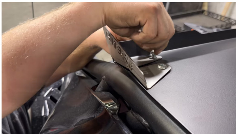
FIG 9 - Fasten the rear wings to the vehicle
