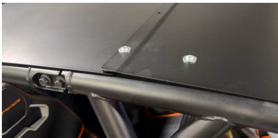
FIG 8 - Loosley fasten center sides of roof halves to vehicle
