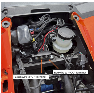
FIG 4 & FIG 5 - Connect the Black, White, and Blue wires to the switch. Connect the ring terminals of the harness to the under hood busbar
