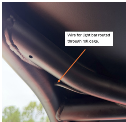
FIG 3 - Route the light bar wire through the roll cage
