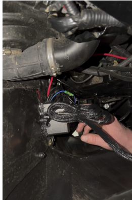
FIG 18 - Fasten the winch contactor box to the inside of the rear passenger wheel
