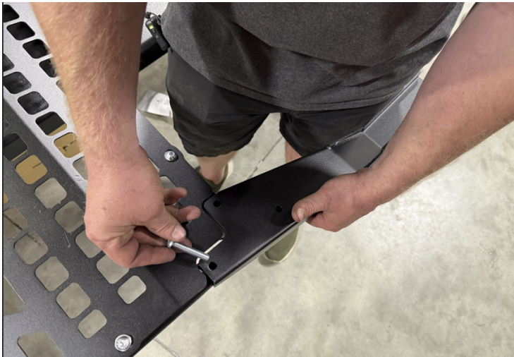
FIG 11 - Fasten the lower mount brackets to the headache rack frame
