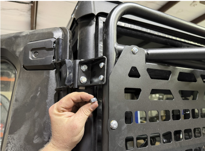
FIG 13 - Use the M8 hardware to fasten the headache rack to the upper mount brackets
