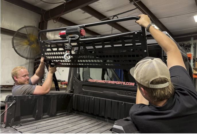
FIG 12 - Hang the headache rack frame from the upper mount brackets
