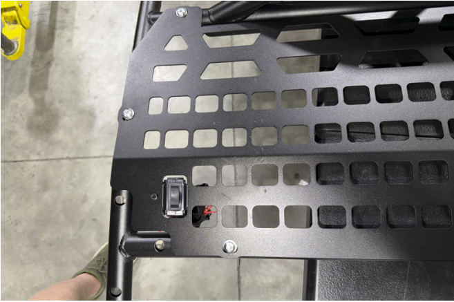
FIG 6 - Fasten the manual switch to the rear panel
