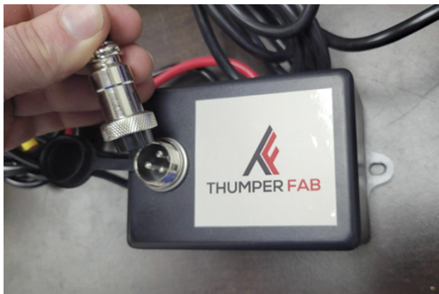
FIG 16 - Plug manual switch harness into winch contactor box
