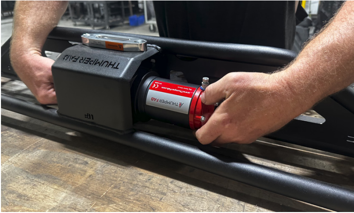
FIG 8 - Fasten the winch to the headache rack frame
