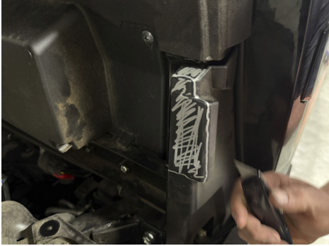
FIG 1 & FIG 2 - Trim the plastics for the lower cab mounts
