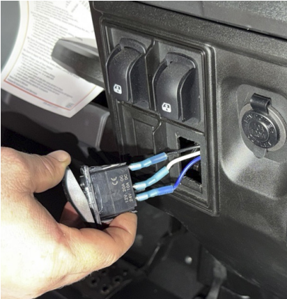
FIG 22 & FIG 23 - Connect the harness to the switch and insert switch in dash
