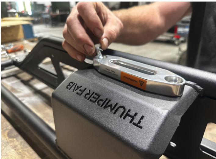
FIG 7 - Fasten the fairlead to the headache rack frame
