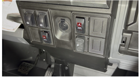
FIG 22 & FIG 23 - Connect the harness to the switch and insert switch in dash
