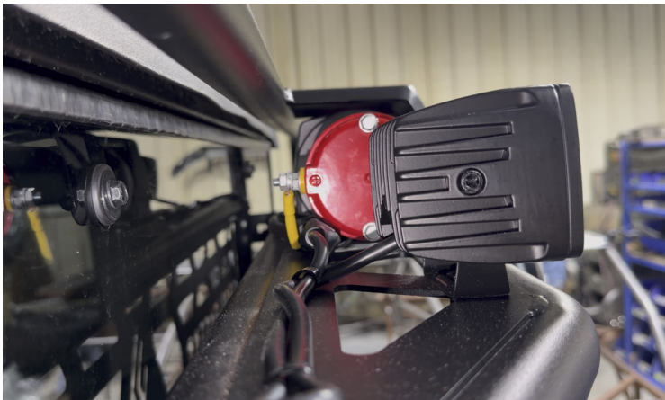
FIG 17 - Connect winch and manual switch to contactor box
