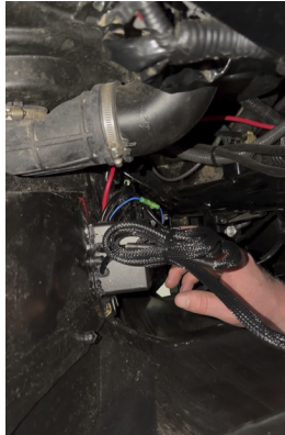
FIG 16 - Fasten the winch contactor box to the inside of the rear passenger wheel
