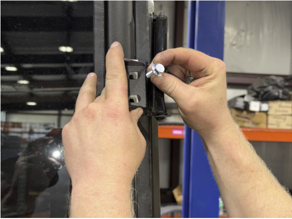
FIG 10 - Loosely fasten the upper mount brackets to the vehicle
