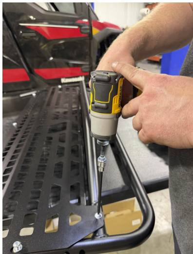
FIG 5 - Fasten rear panel to headache rack frame
