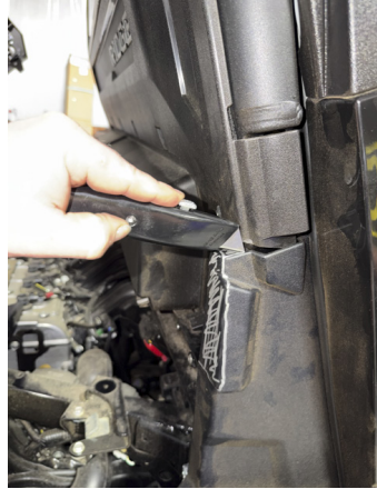
FIG 1 & FIG 2 - Trim the plastics for the lower cab mounts
