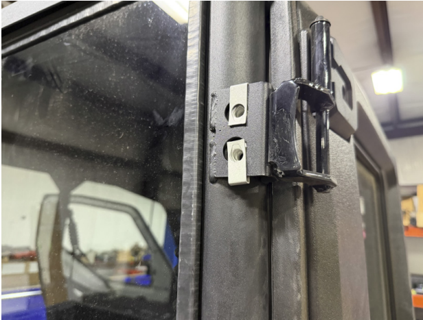
FIG 4 - Install the M8 slip on barrel nuts onto the OEM roll cage brackets
