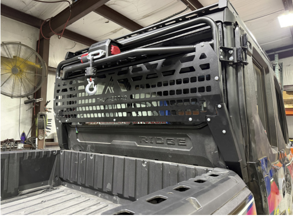
FIG 14 - Fasten the lower mount brackets to the frame. Tighten all hardware
