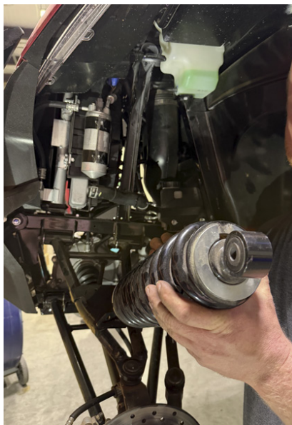
FIG 2 - Remove the front shock upper mounting bolt
