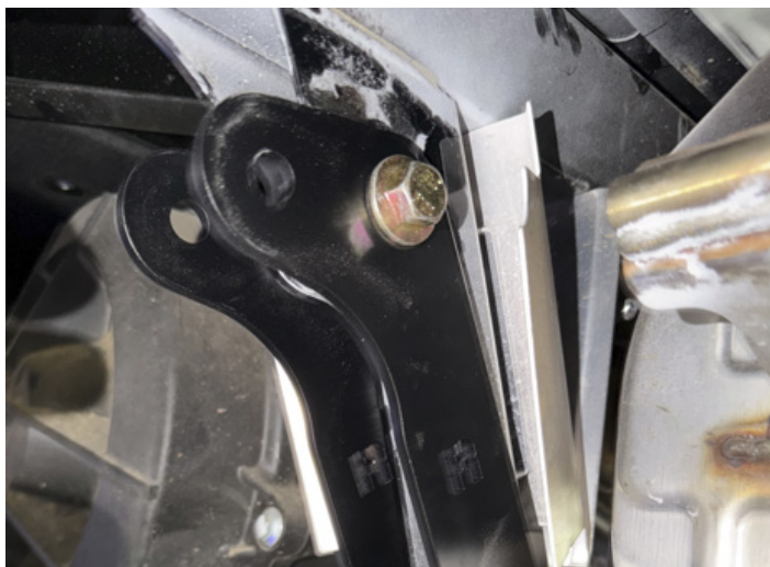
FIG 8 - Fasten rear shock brackets to the rear frame section
