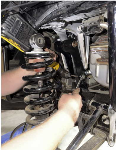
FIG 10 - Tighten remaining rear shock lift bracket hardware
