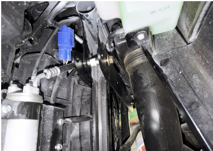
FIG 4 - Loosley mount the front driver and passenger lift brackets
