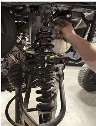
FIG 7 - Disconnect the rear shock from the frame
