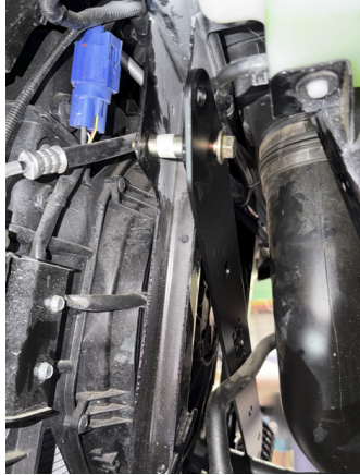
FIG 3 - Loosley fasten the front main lift bracket to the frame
