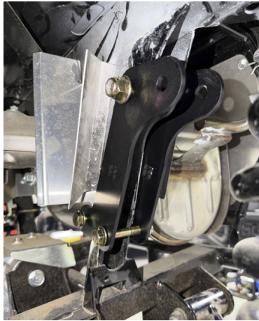
FIG 9 - Fasten the rear lift brackets to the frame
