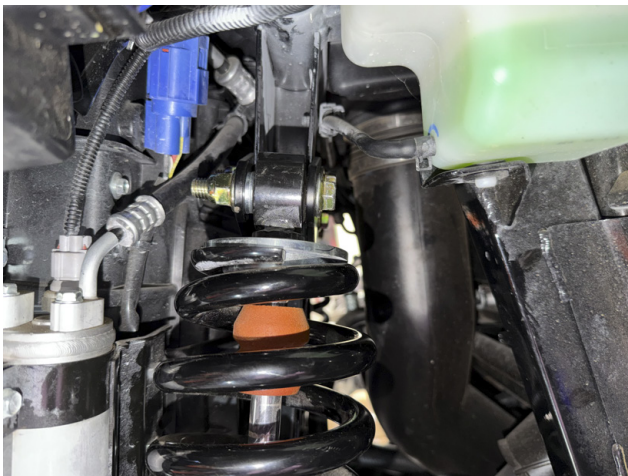
FIG 6 - Fasten front shock to the front lift brackets
