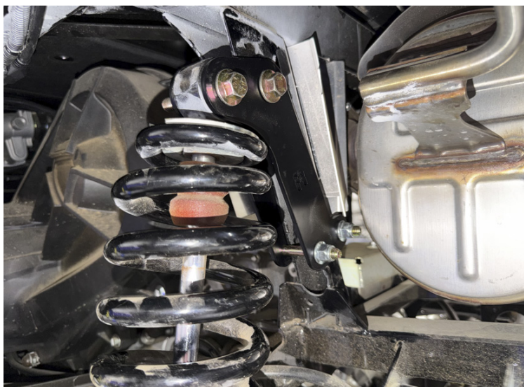
FIG 11 & FIG 12 - Fasten the rear shock to the rear lift brackets
