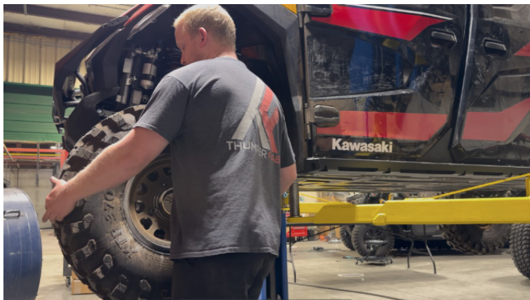
FIG 1 - Lift the vehicle in the air and remove the wheels
