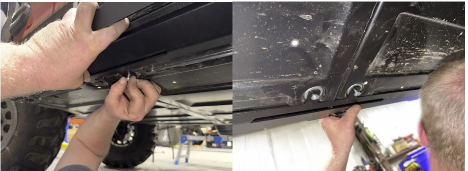
FIG 18 & FIG 19 - Loosley mount the lower nerf rail body to the underside of the vehicle
