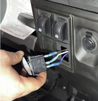
FIG 17 & FIG 18 - Connect the harness to the switch and insert switch in dash
