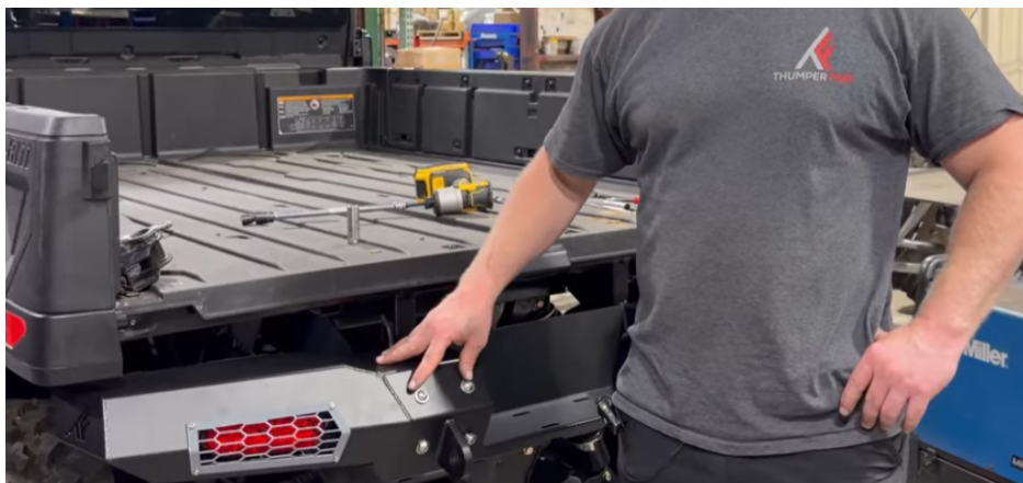
FIG 12 - Mount the bumper body to the mount brackets
