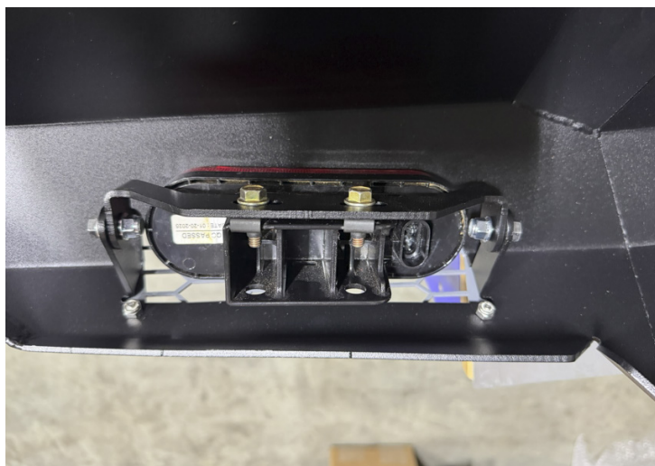
FIG 6 - Fasten OEM tail lights to Bumper Body
