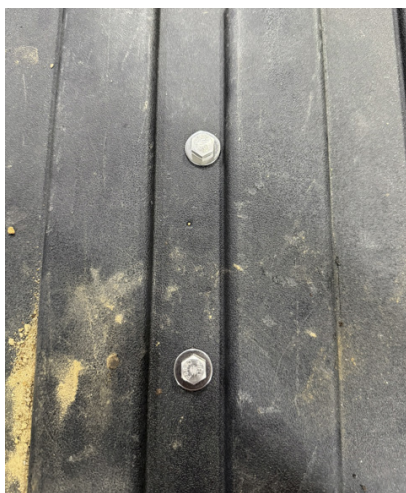
FIG 14 - Fasten the remaining mount holes to the bed through the drilled holes
