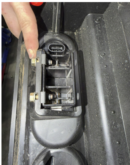
FIG 3 - Remove tail lights from OEM tail light rear panel
