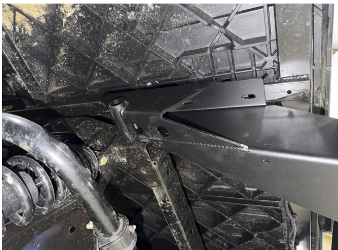
FIG 10 - Slide the mount brackets into place over the frame pivot tube
