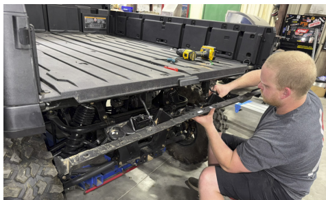
FIG 1 & FIG 2 - Unplug and remove tail light panel assembly
