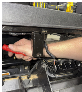
FIG 1 & FIG 2 - Unplug and remove tail light panel assembly
