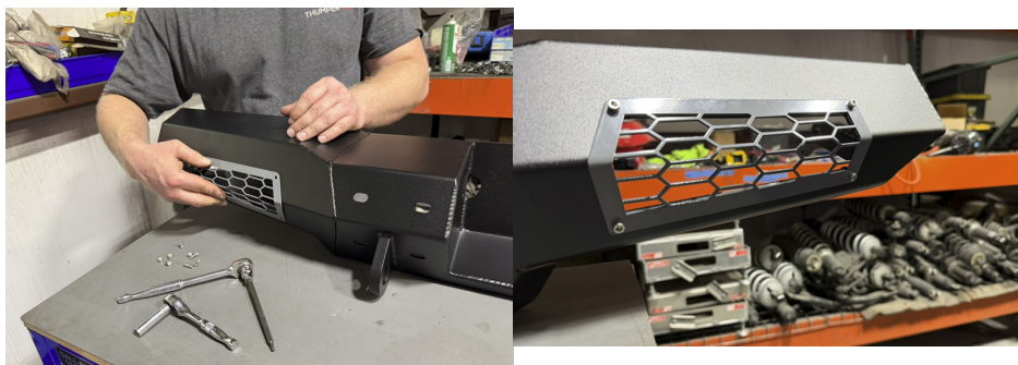
FIG 4 & FIG 5 - Mount Light Covers to Bumper Body
