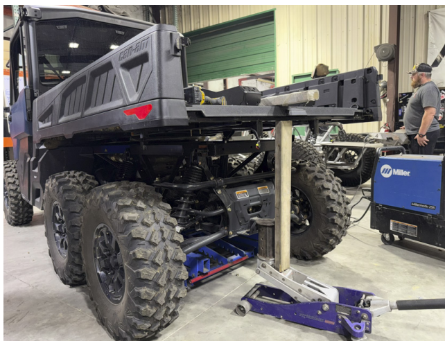
FIG 8 - Disconnect bed tilt actuator and jack up rear of bed
