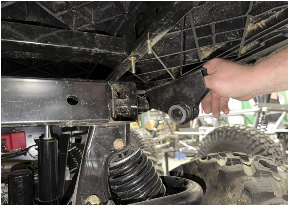
FIG 9 - Remove bed pivot brackets
