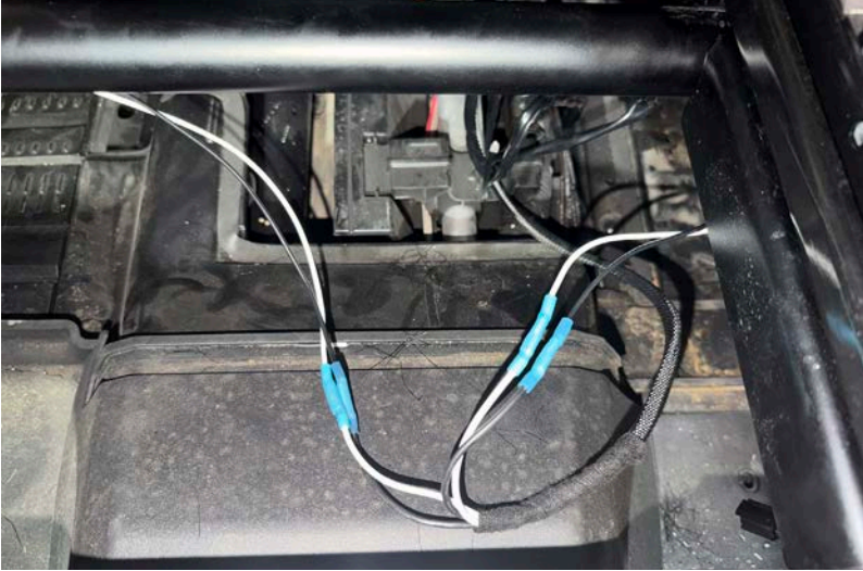
Seat Heater Wiring
