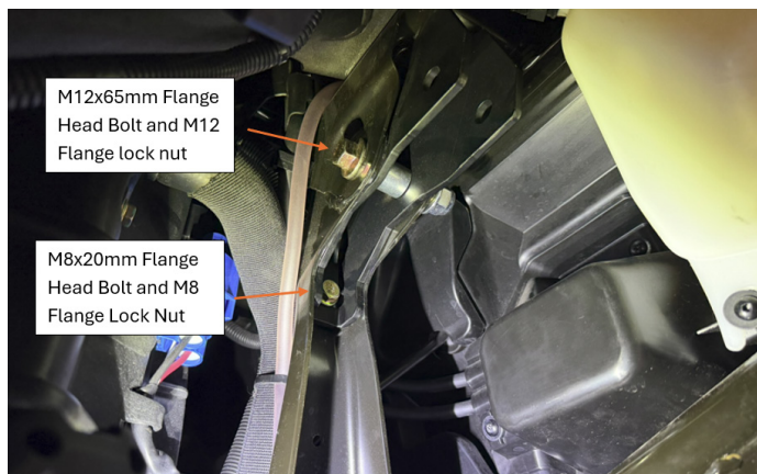
FIG 4 - Fasten the front lift brackets to the vehicle
