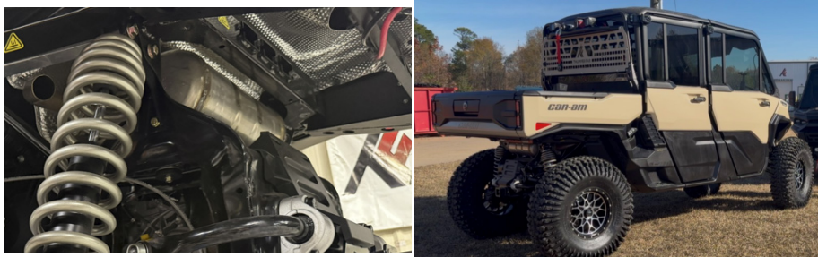
FIG 8 & FIG 9 - Fasten the rear shock to the rear lift bracket and rear lower control arm
