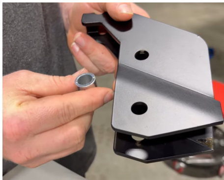
FIG 2 & FIG 3 - Insert the spacers between the flanges of the lift brackets
