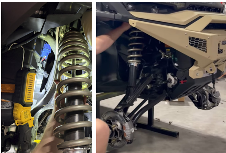
FIG 5 & FIG 6 - Fasten the front shock to the front lift bracket and front upper control arm
