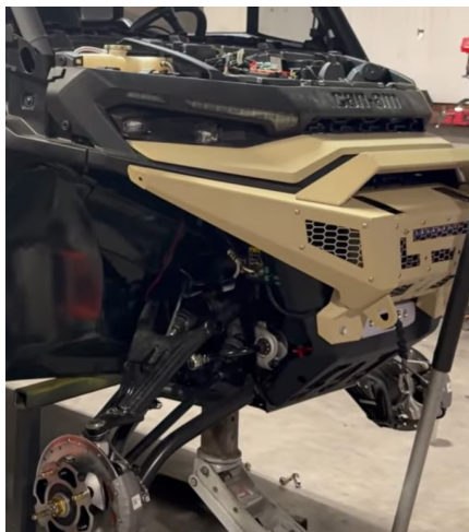
FIG 1 - Remove the front and rear shocks and set aside
