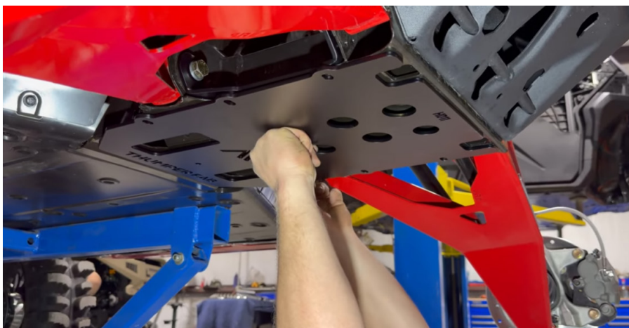
FIG 9 - Loosley fasten center of the main plate to the underside of the frame
