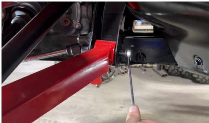
FIG 1 - Remove the lower control arm mounting hardware
