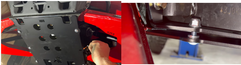
FIG 7 & FIG 8 - Loosley fasten the Middle Support Brackets to the Main Plate
