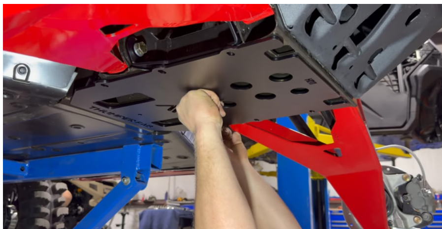
FIG 6 - Loosley fasten main plate to the underside of the vehicle
