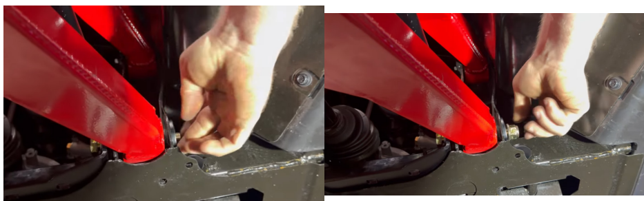
FIG 4 & FIG 5 - Loosley fasten the Rear Support Brackets to the Frame
