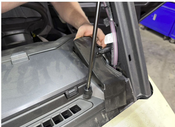
FIG 15 - Remove Dash Closeout Panel
