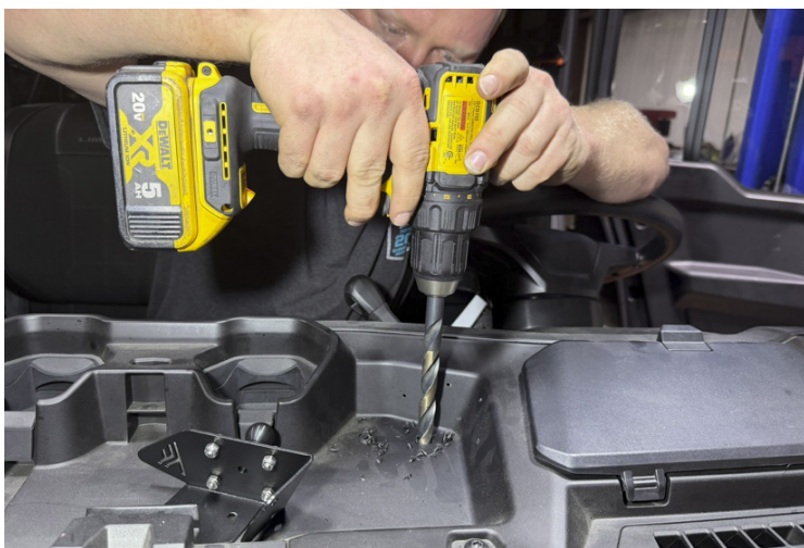
FIG 7 - Drill hole for wiring (IF INSTALLING WIRELESS PHONE CHARGER)
