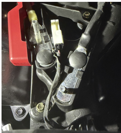
FIG 18 - Connect harness to busbar
