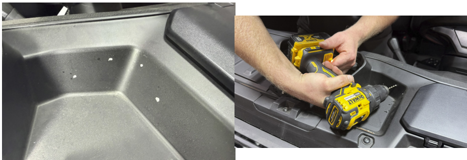
FIG 5 & FIG 6 - Drill pilot holes
