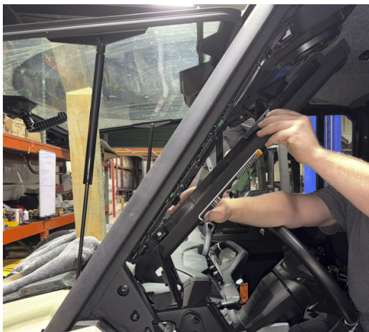
FIG 14 - Remove A-Pillar Plastic Tunnel
