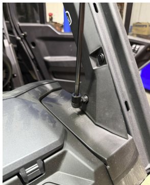
FIG 11 - Disconnect Windshield Struts from A-Pillar Mount
