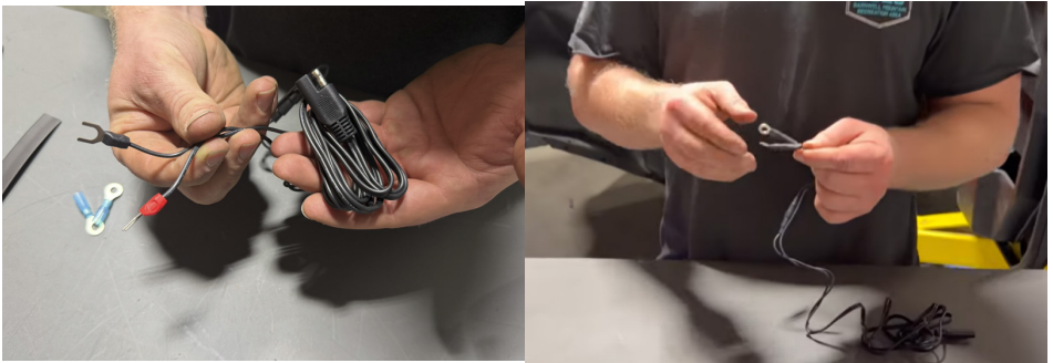
FIG 9 & FIG 10 - Replace connectors on harness with 1/4" ring terminals
