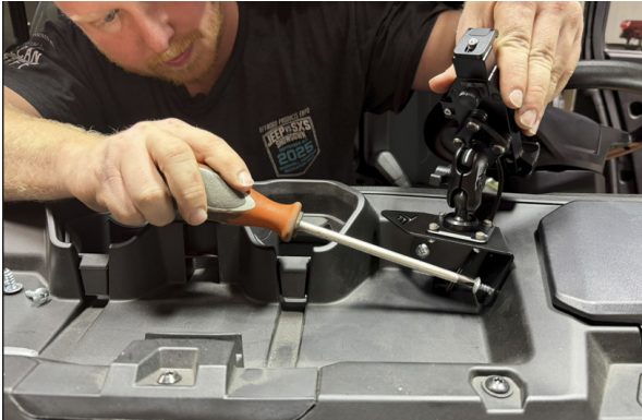
FIG 8 - Mount bracket assembly to dash
