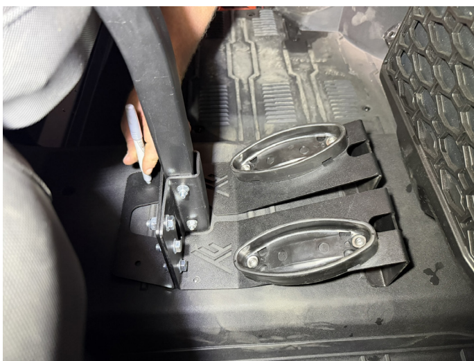
FIG 6 - Mark mounting holes
