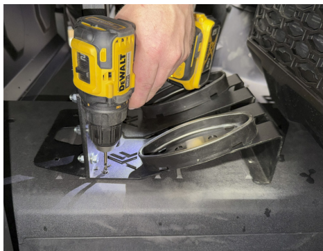
FIG 7 - Drill pilot holes for mounting screws
