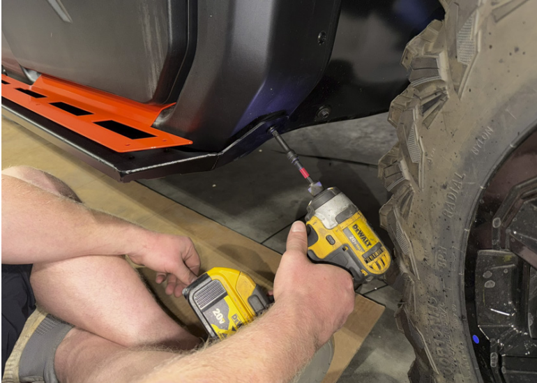
FIG 6 - Fasten front of bottom body to vehicle
