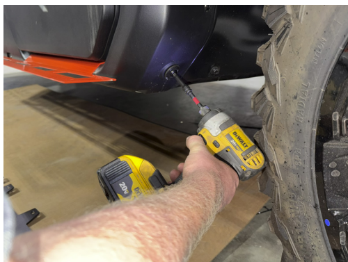
FIG 3 - Remove the OEM fender well bolt
