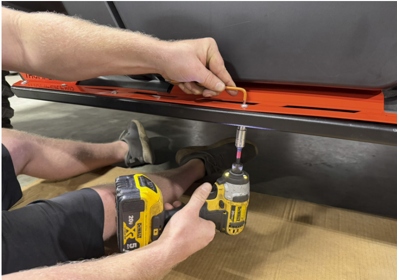
FIG 10 - Install the remaining fasteners and tighten all hardware
