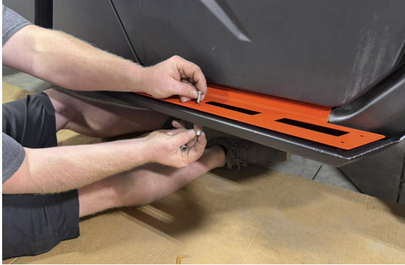
FIG 7 - Fasten nerf rail top and bottom bodies together
