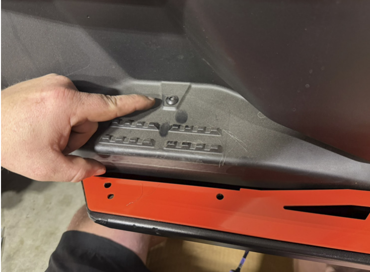
FIG 8 - Remove OEM fastener from rear quarter panel
