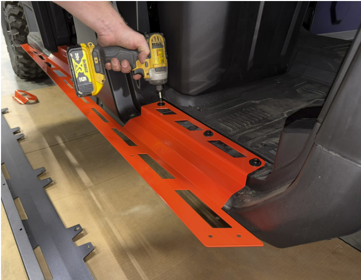
FIG 2 - Mount the Top Body to the Vehicle
