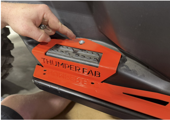
FIG 9 - Fasten rear mount bracket to vehicle
