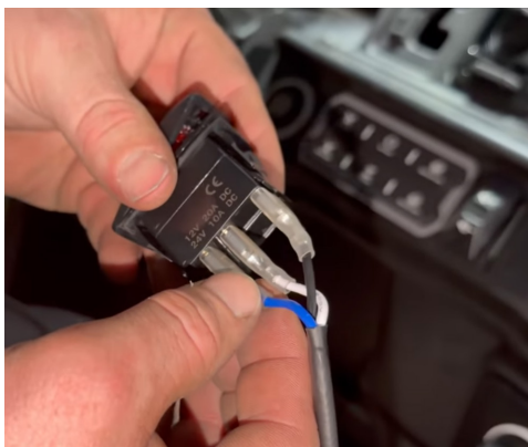
FIG 36 - Connect Harness to Switch
