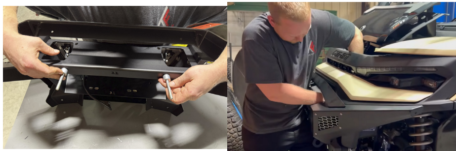
FIG 22 & FIG 23 - Loosely fasten the top portion of the bumper to the vehicle
