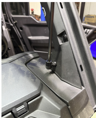
FIG 26 - Disconnect Windshield Struts from A-Pillar Mount
