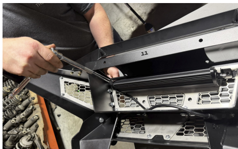
FIG 13 & FIG 14 - Mount light to Bumper (IF LIGHT OPTION WAS SELECTED)
