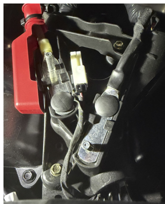
FIG 33 & FIG 34 - Connect Harness to Busbar
