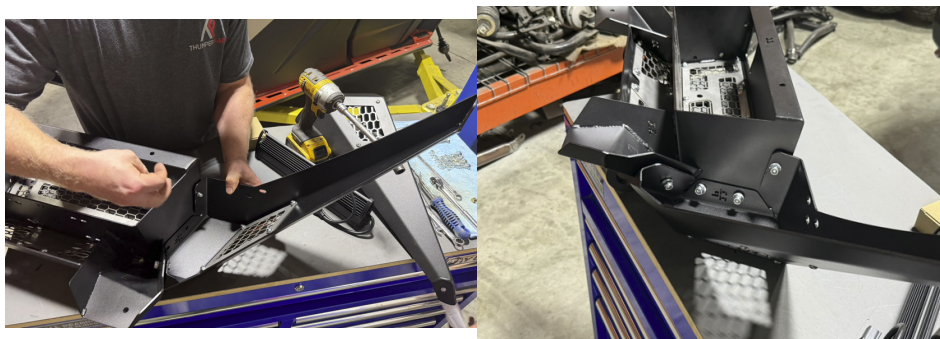
FIG 9 & FIG 10 - Fasten Wings to Main Bumper Shell
