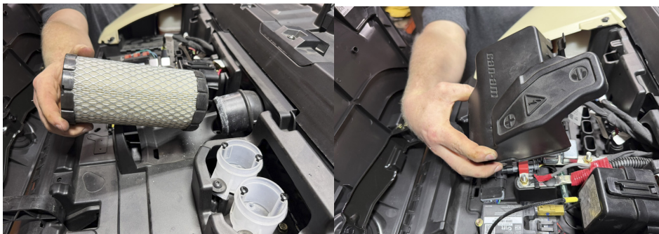
FIG 17 & FIG 18 - Remove cabin air filter and jump start cover
