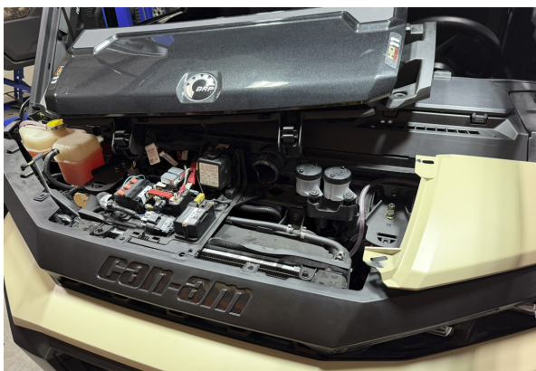
FIG 35 - Route wires to light bar and plug light bar into harness
