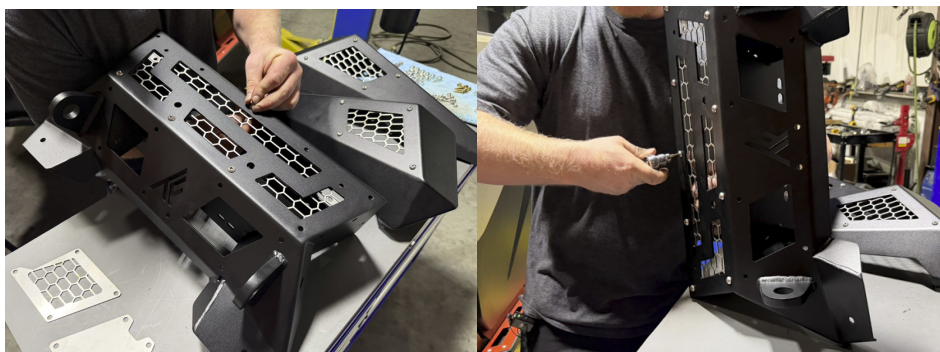
FIG 5 & FIG 6 - Fasten Upper Accent Panel to Main Bumper Shell
