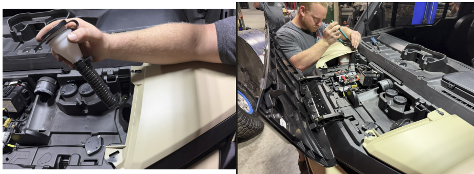
FIG 19 & FIG 20 - Remove the wiper fluid filler neck and tray mounting bolts
