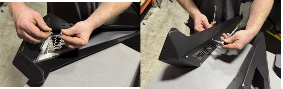
FIG 1 & FIG 2 - Fasten Wing Accent Panels to Wings
