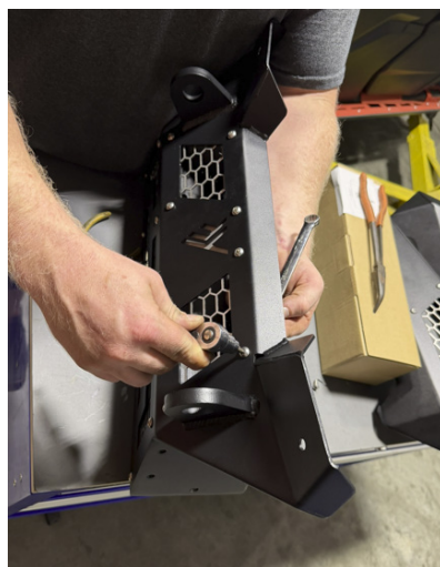
FIG 7 & FIG 8 - Fasten Logo and Lower Accent Panels to Bumper Shell
