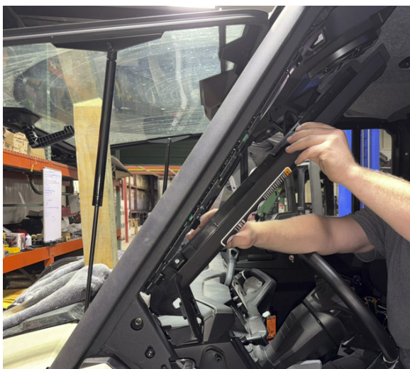
FIG 29 - Remove A-Pillar Plastic Tunnel
