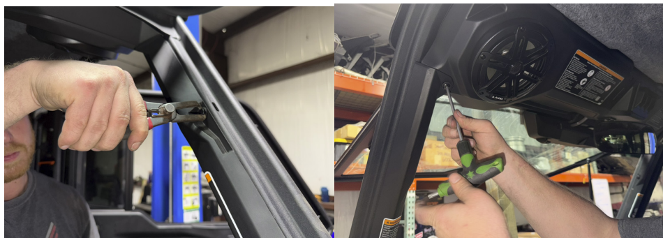
FIG 27 & FIG 28 - Remove fasteners holding A-Pillar plastic tunnel to vehicle
