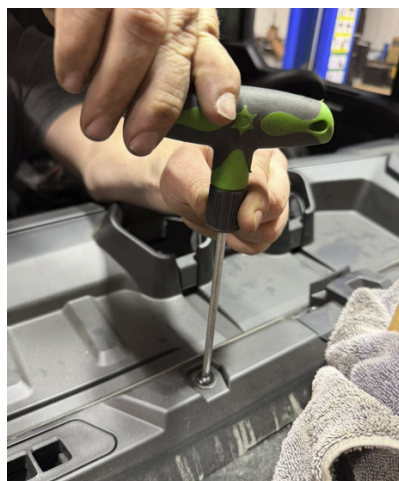
FIG 31 & FIG 32 - Remove dash pad fasteners
