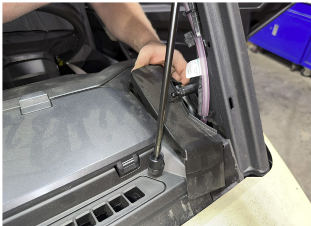
FIG 30 - Remove Dash Closeout Panel
