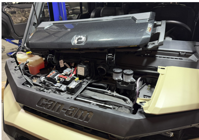
FIG 21 - Remove the hood and underhood tray from the vehicle
