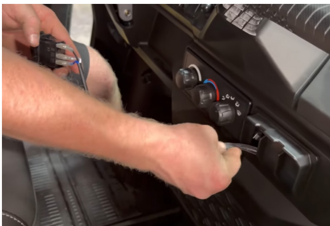
FIG 37 - Snap switch into dash and test lights
