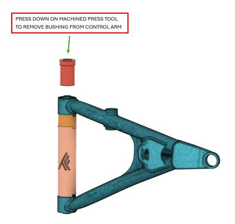
FIG 2 - Remove bushings from OEM control arms
