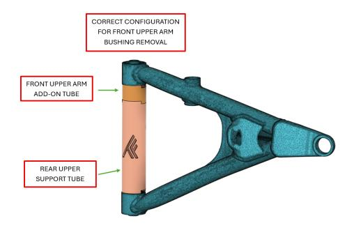
FIG 1 - Select correct configuration of support tubes
