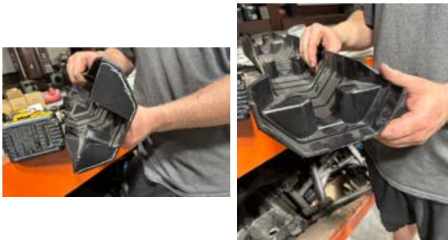
FIG 19 & FIG 20 - Mark and cut Middle Cross Bar Plastic Guard
