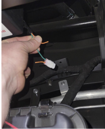
FIG 17 - Orange and red wire - Key On Power
