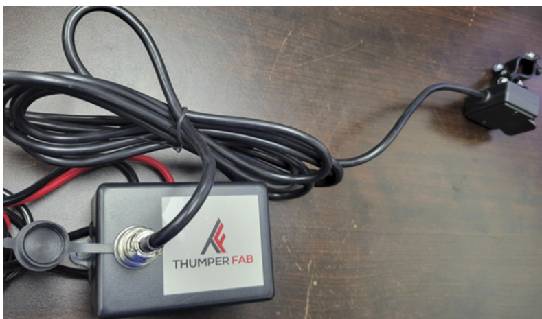
FIG 16 - Tighten switch harness to contactor box
