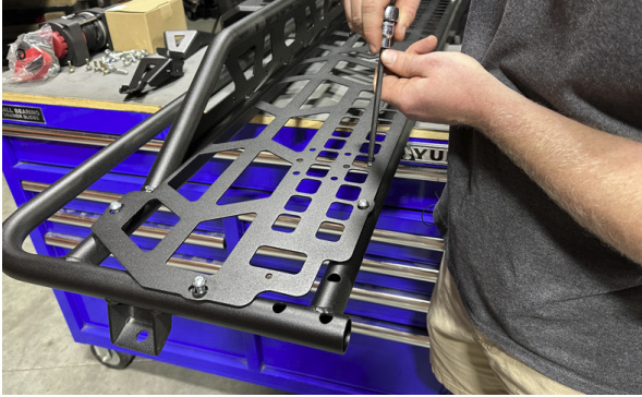
FIG 1 - Fasten Rear Panel to Headache Rack Frame
