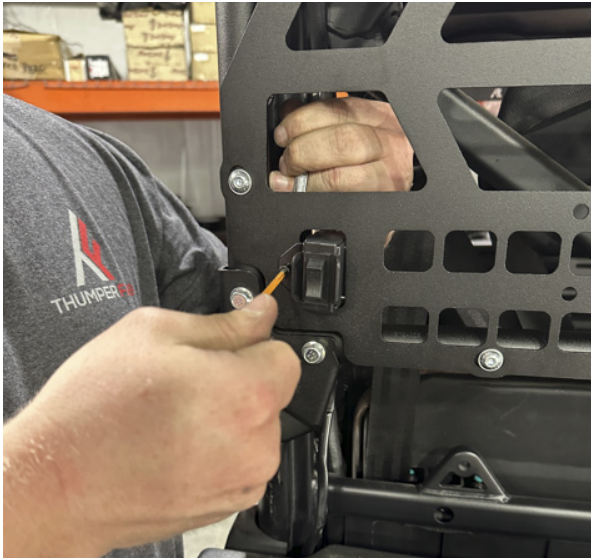
FIG 6 - Mount the Winch Switch to the Rear Panel
