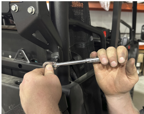
FIG 12 - Tighten Frame Mounting bolts using a 13mm Socket
