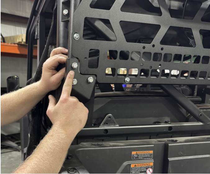
FIG 11 - Fasten Lower Brackets to Headache Rack Frame
