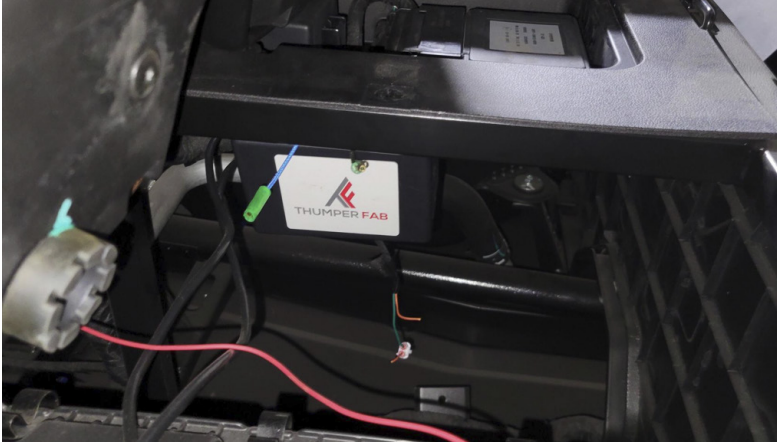
FIG 13 - Mount Contactor Box using Truss Screws
