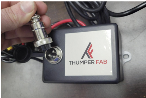
FIG 15 - Plug manual switch harness into winch contactor box
