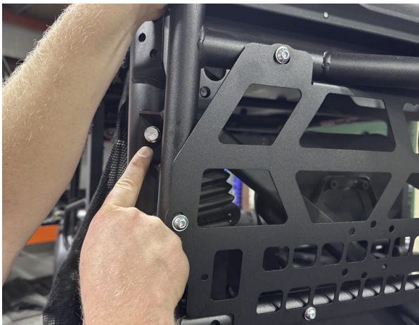
FIG 10 - Fasten the Headache Rack to the Vehicle
