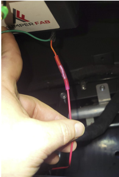
FIG 18 - Splice wires together
