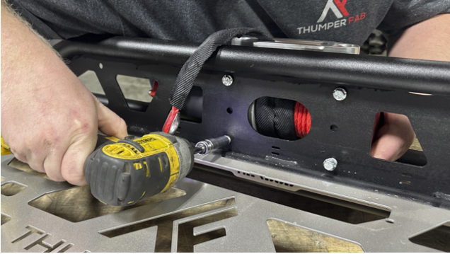
FIG 3 - Fasten Winch to Headache Rack Frame
