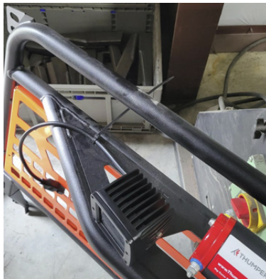
FIG 8 - Fasten the Cube Light to the Headache Rack Frame
