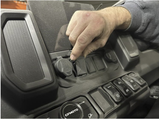
FIG 21 - Remove Switch Cover
