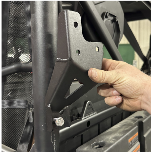
FIG 9 - Loosley Fasten Lower Brackets to Vehicle
