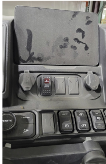
FIG 22 & FIG 23 - Wire switch and install into Dash
