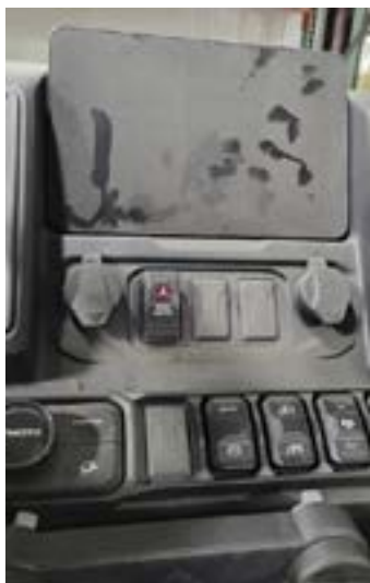
FIG 19 & FIG 20 - Wire switch and install into Dash
