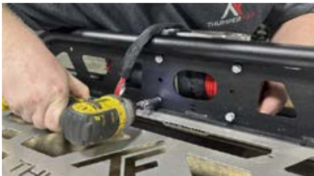
FIG 3 - Fasten Winch to Headache Rack Frame
