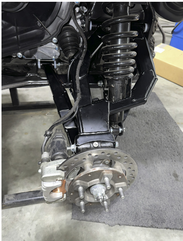
FIG 10 - Zip tie Brake Line and Parking Brake Cable to Upper Control Arms
