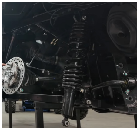
FIG 1 - Remove OEM Control Arms
