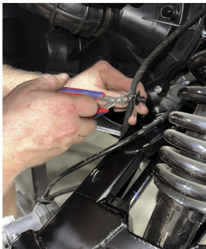
FIG 8 & FIG 9 - Remove OEM brake line clamps
