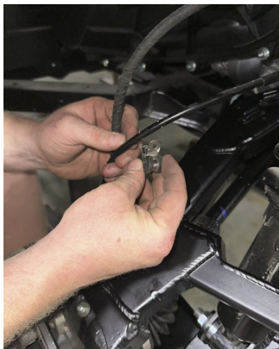
FIG 8 & FIG 9 - Remove OEM brake line clamps
