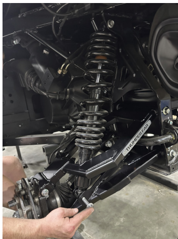
FIG 5 - Mount the shock to the Lower Control Arm
