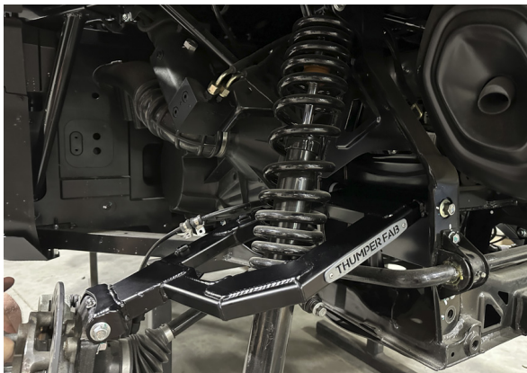
FIG 2 - Fasten Upper Control Arm to vehicle
