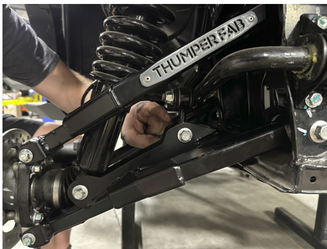
FIG 6 - Attach the sway bar to the Lower Control Arm
