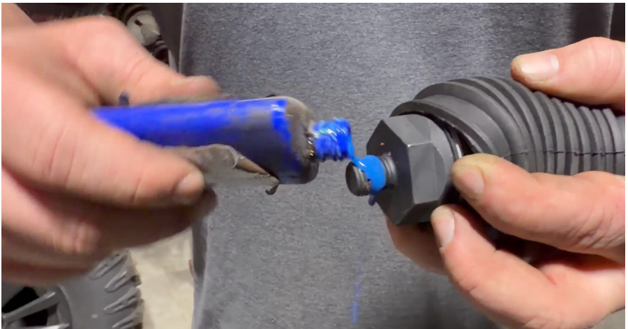
FIG 9 - Apply loctite to the inner tie rod
