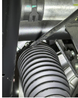
FIG 1 & FIG 2 - Remove OEM steering boot clamp
