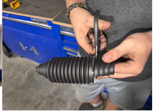
FIG 4 & FIG 5 - Trim the new steering boot
