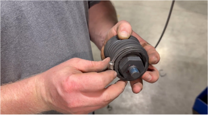
FIG 10 - Slide hose clamp over steering boot
