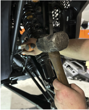
FIG 1 & FIG 2 - Remove OEM steering boot clamp
