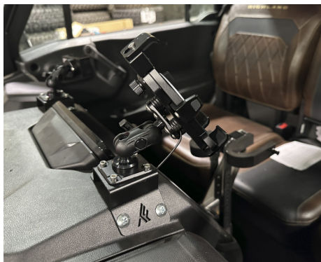
FIG 11 & FIG 12 - Fasten Mount Bracket to the Dash
