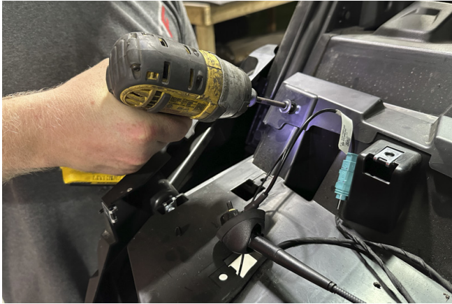
FIG 8 - Remove 5 X OEM screws with T30 Torx
