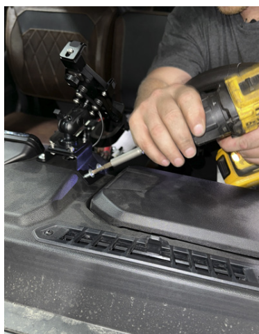
FIG 11 & FIG 12 - Fasten Mount Bracket to the Dash
