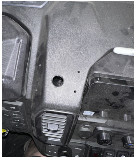
FIG 7 - Clean hole with Deburring Tool
