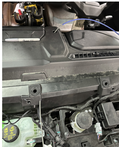
FIG 9 - Route wiring to the Hood Section of Vehicle
