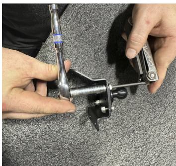
FIG 1 - Fasten Ball Mount to Mount Bracket
