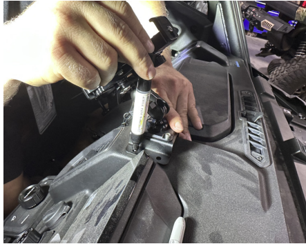
FIG 3 - Mark holes to be drilled
