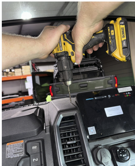
FIG 4 - Drill Marked Holes
