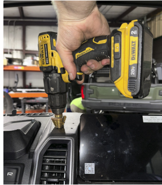
FIG 5 & FIG 6 - Drill hole for Wiring Harness (CHARGING INSTALL ONLY!)
