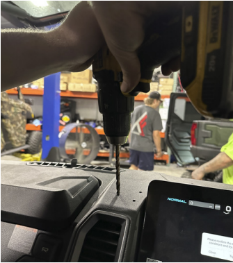
FIG 5 & FIG 6 - Drill hole for Wiring Harness (CHARGING INSTALL ONLY!)
