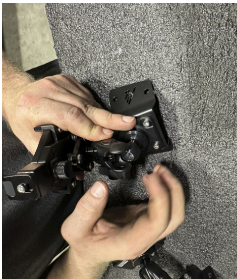
FIG 2 - Assemble Adjustable Swivel Mount and Phone Charging Unit
