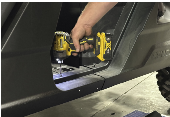
FIG 1 - Remove OEM Bolts using T30 Torx
