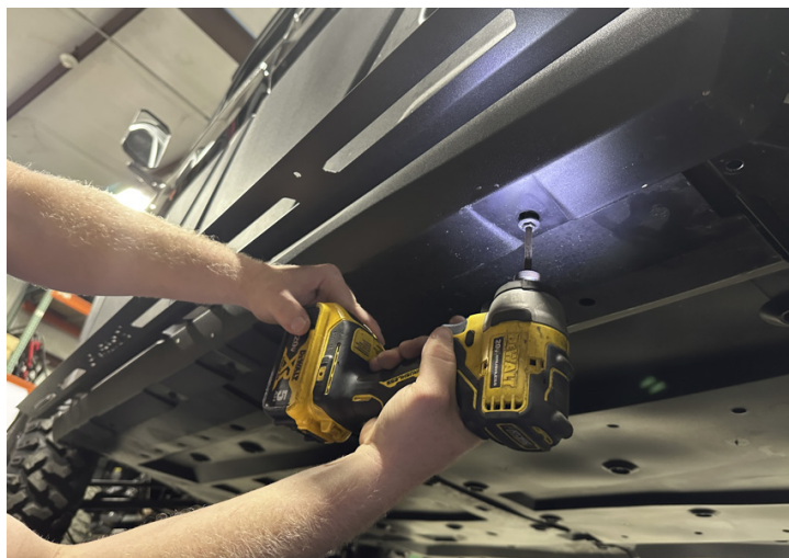
FIG 5 - Remove OEM Skid Plate Outer Bolts
