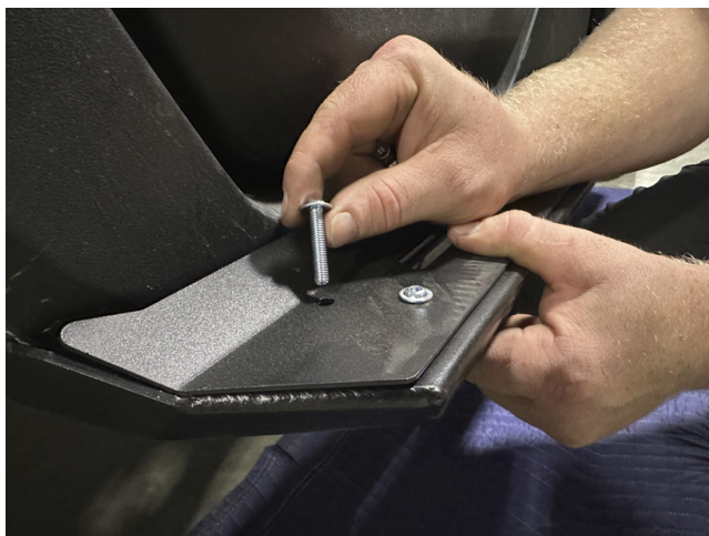
FIG 9 - Fasten Nerf Rail bodies together. Tighten all hardware
