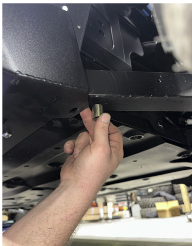
FIG 7 - Put Spacer in Place
