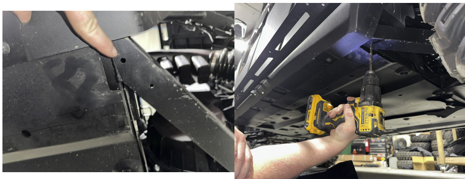
FIG 3 & FIG 4 - Drill hole through Rear Frame Tube
