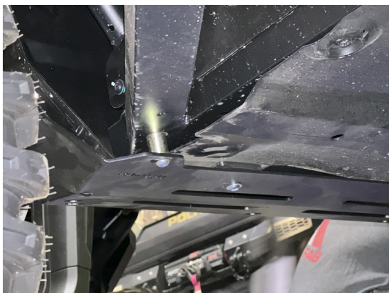
FIG 8 - Fasten Rear of Nerf Rail to Frame
