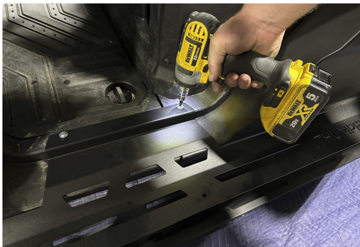
FIG 2 - Mount Upper Nerf Rail Body to Vehicle
