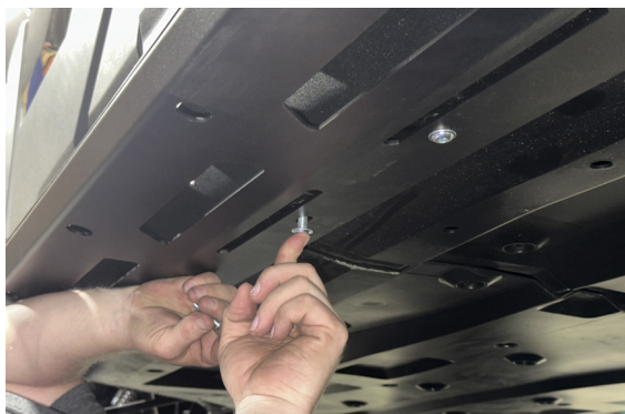
FIG 6 - Fasten Nerf Rail Lower Body
