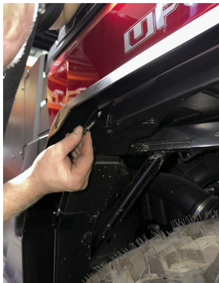
FIG 6 - Mount Rear Fender Flares to vehicle
