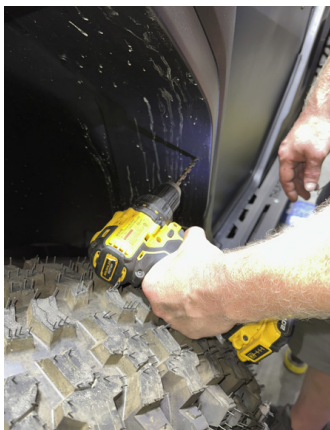
FIG 3 - Drill Marked holes for Front Fender Flares
