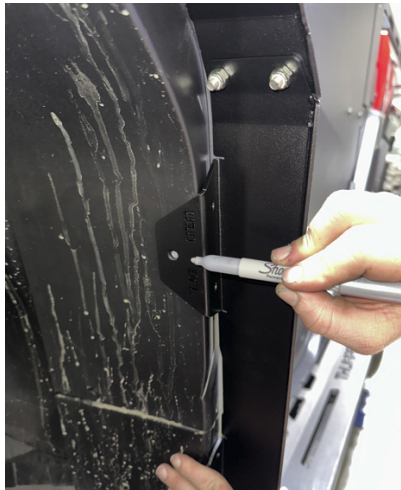
FIG 2 - Mark the front fender flare mounting holes
