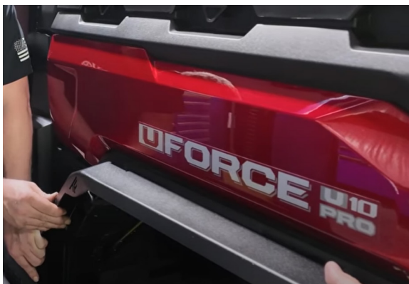
FIG 5 - Mark and Drill holes for Rear fender flares
