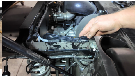
FIG 25 & FIG 26 - Route Contactor Winch Wires to Junction Block
