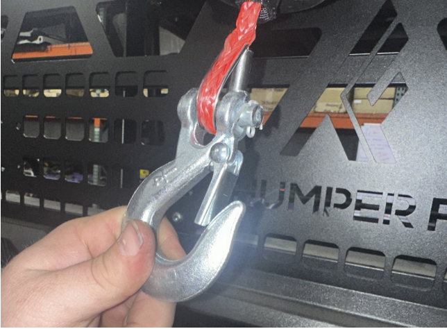
FIG 11 - Mount Winch Hook to the Winch Cable
