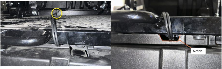
FIG 22 & FIG 23 - Notch Plastic and route Extension Wires to the front of the bed frame
