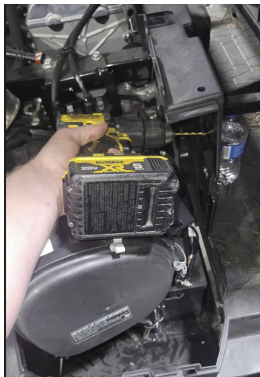
FIG 15 - Locate and drill contactor box mount holes
