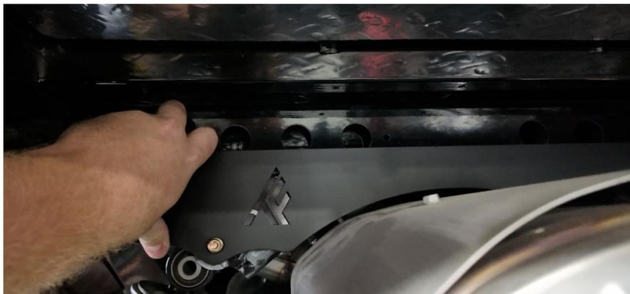
**FIG 3 - Mount Rear Lift Brackets to Frame**
