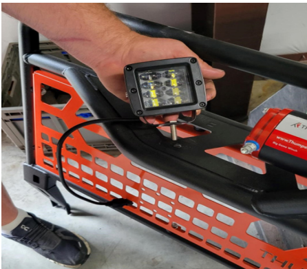
FIG 18 - Fasten Cube Light to Headache Rack
