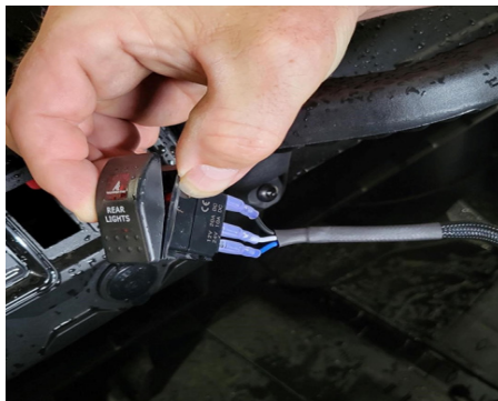
FIG 19 - Select slot for switch, check wiring before installation. Snap switch into slot in dash.
