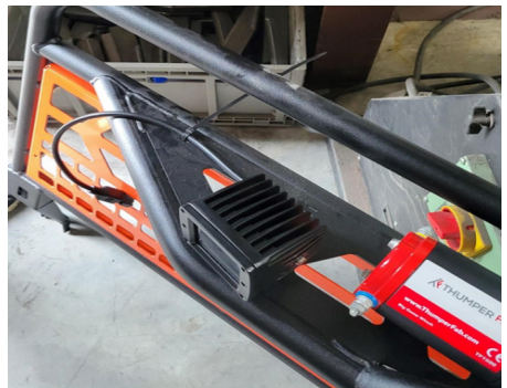
FIG 19 - Ziptie Cube Light Pigtail to Headache Rack
