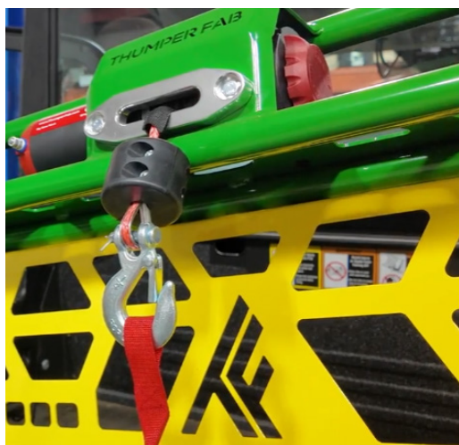
FIG 13 - Fasten Winch Stop and Winch Hook to the Winch Cable
