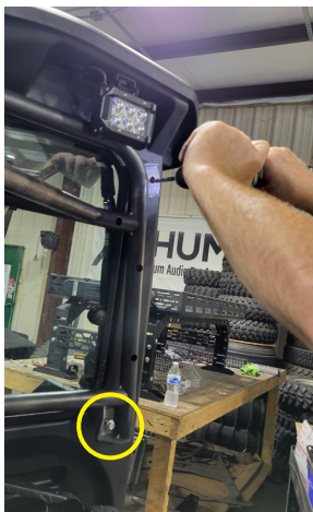
FIG 2 - Drill upper holes through rear panel using a 3/8" Drill Bit
