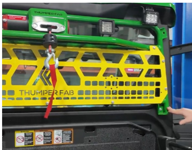
FIG 15 - Fasten Headache Rack Lower Mounts to Vehicle
