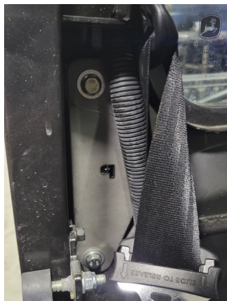
FIG 7 & FIG 8 - Mount Lower Driver and Passenger Inner Brackets
