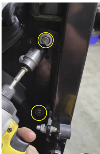
FIG 5 & FIG 6 - Remove OEM Flange Head Bolts and set aside
