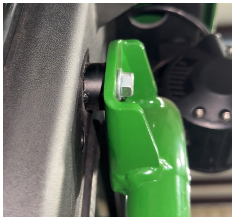
FIG 16 - Mount the Headache Rack Upper Mounts to the vehicle
