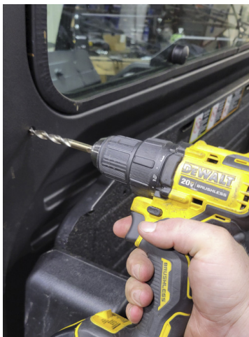
FIG 1 - Drill lower holes through rear panel using a 3/8" Drill Bit
