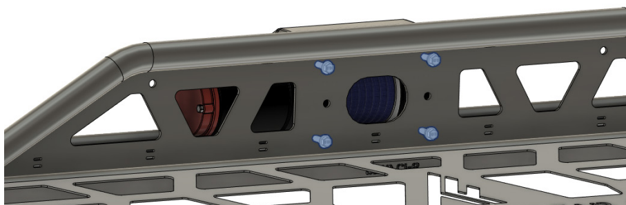
FIG 11 - Fasten Fairlead to Headache Rack Frame
