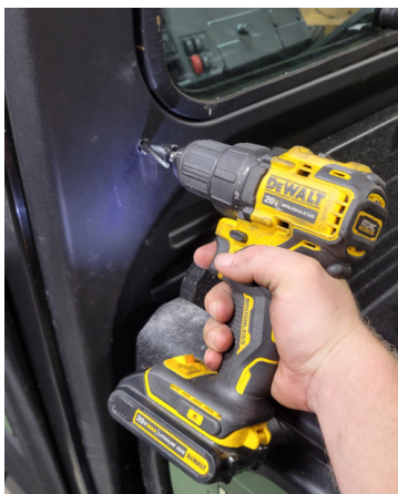
FIG 3 & FIG 4 - Drill lower holes through rear panel using a 3/4" Drill Bit or a Step Up Bit
