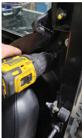
FIG 3 & FIG 4 - Drill lower holes through rear panel using a 3/4" Drill Bit or a Step Up Bit
