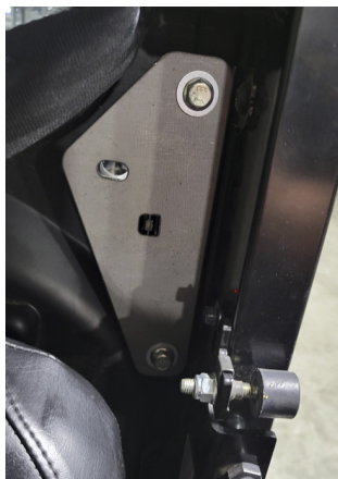
FIG 7 & FIG 8 - Mount Lower Driver and Passenger Inner Brackets
