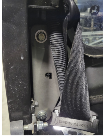
FIG 7 & FIG 8 - Mount Lower Driver and Passenger Inner Brackets
