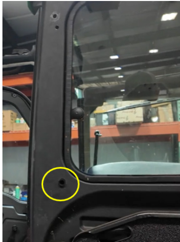
FIG 9 - Insert Lower Spacers through Rear Panel
