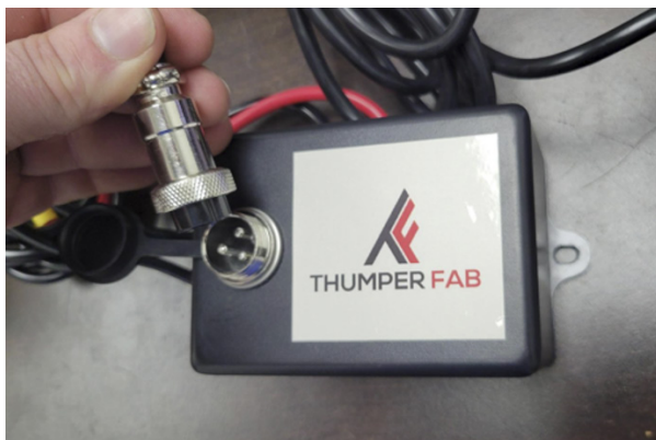
FIG 18 - Plug manual switch harness into winch contactor box
