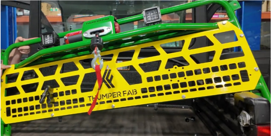
FIG 14 - Mount the Cube Lights to the Headache Rack Frame (OPTIONAL)
