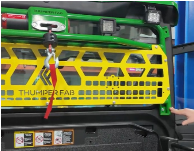
FIG 15 - Fasten Headache Rack Lower Mounts to Vehicle
