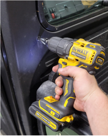
FIG 3 & FIG 4 - Drill lower holes through rear panel using a 3/4" Drill Bit or a Step Up Bit
