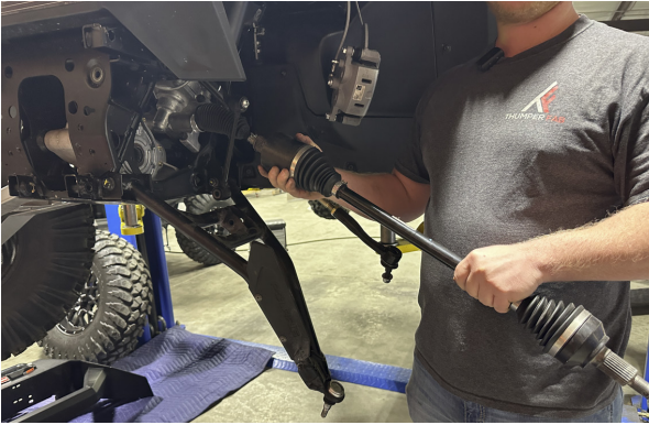
FIG 1 - Remove OEM Suspension and Front Bumper
