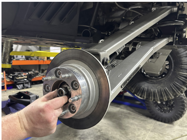
FIG 28 - Install Rear Axle Nut
