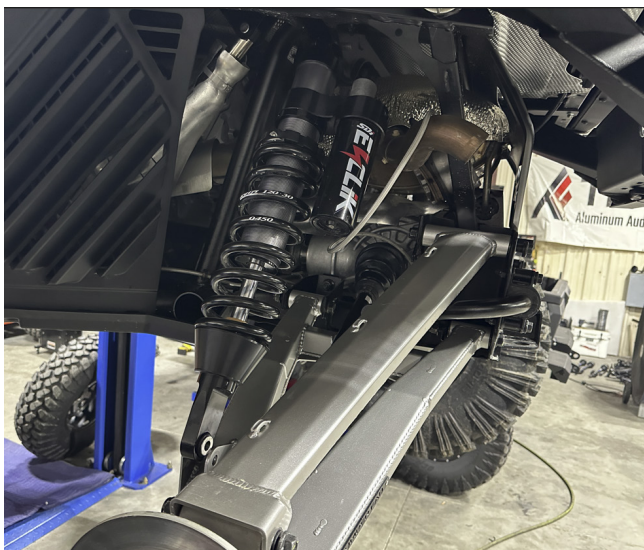
FIG 29 - Mount the Rear Shock to the Frame (Outer Most Hole)
