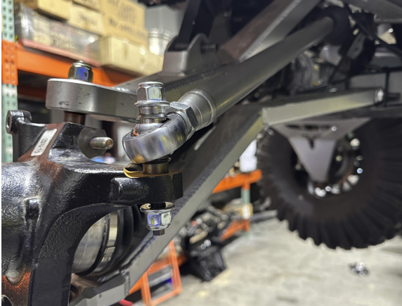
FIG 18 - Mount the tie rod to the knuckle using an 18mm Socket
