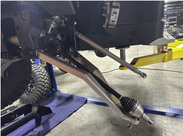
FIG 12 - Install axle into front differential
