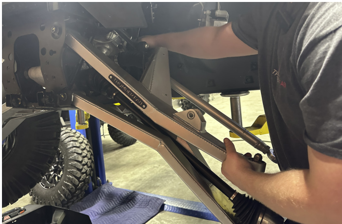
FIG 14 - Install Upper Control Arm using an 18mm Socket and Wrench
