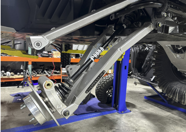
FIG 26 - Install the Rear Axles
