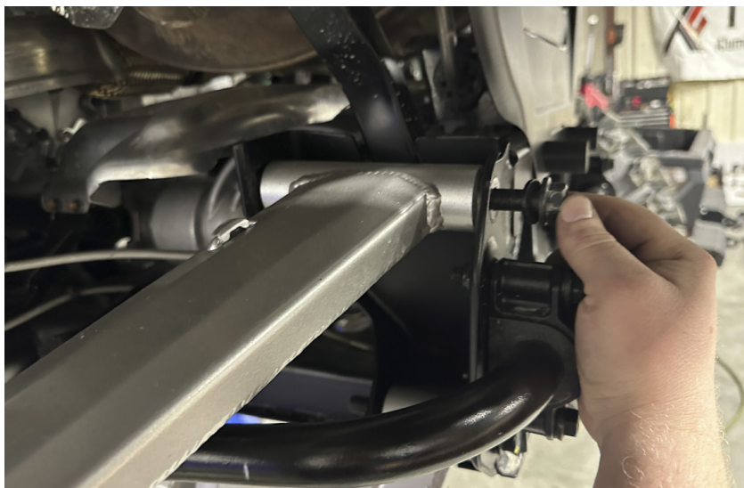
FIG 25 - Mount the Upper Control Arm to the Unit
