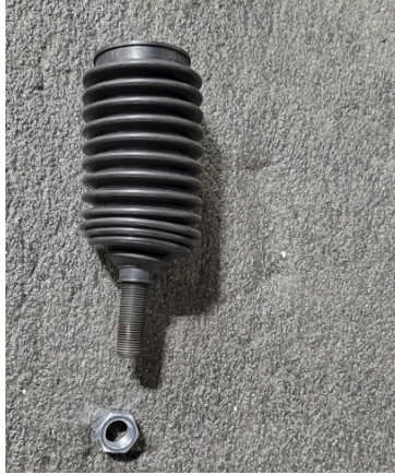
FIG 3 - Slide Inner Tie Rod end through steering rack boot and reinstall jam nut
