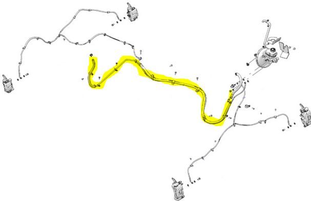
FIG 7 - Replace Brake Lines
