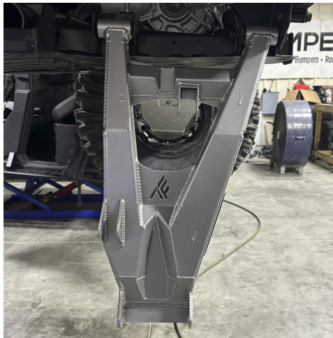
FIG 23 - Mount the Rear Lower Control Arm to the unit
