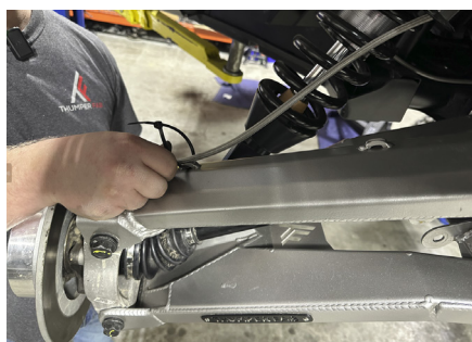
FIG 31 - Fasten the Brake Line to the Upper Control Arm
