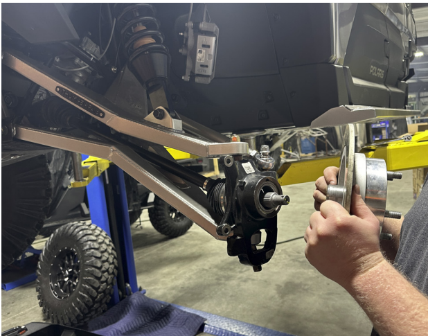
FIG 19 - Mount Rotor to the Knuckle using a 30mm Socket
