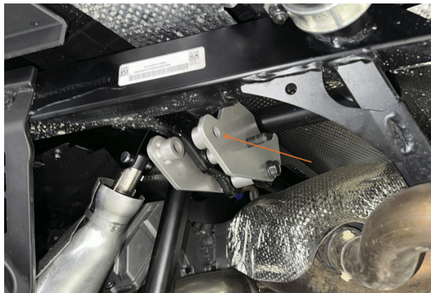
FIG 4 - Relocated Rear Shock Upper Mounting Position
