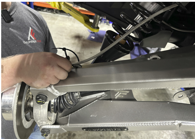
FIG 30 - Mount the sway bar to the lower control arm
