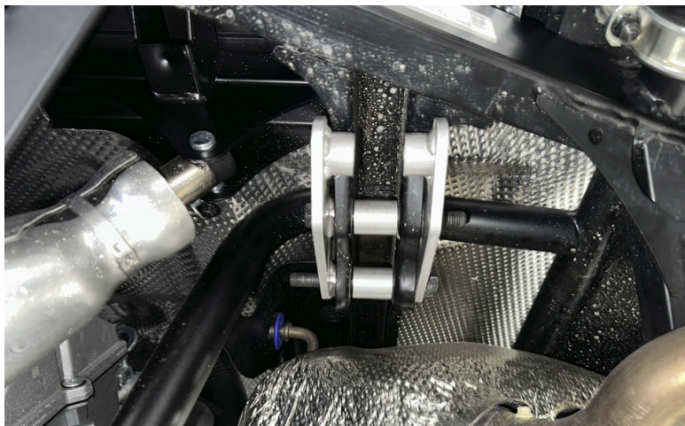
FIG 3 - Mount Rear Shock Relocation Brackets and Spacers to Frame
