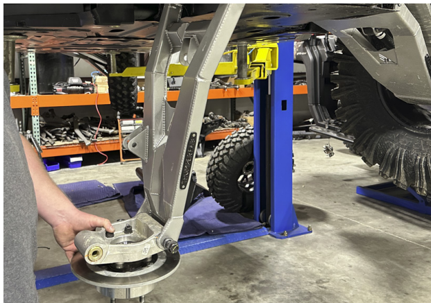
FIG 24 - Mount the knuckle to the lower control arm
