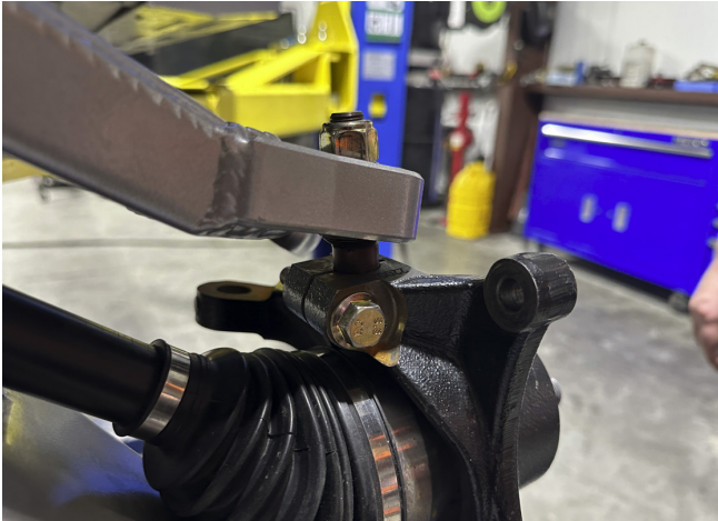
FIG 15 - Mount the knuckle to the Upper Ball Joint using a 15mm Socket and Wrench
