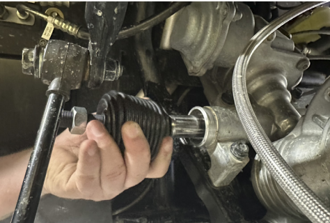
FIG 4 - Fasten Inner Tie Rod to steering rack using Channel Locks
