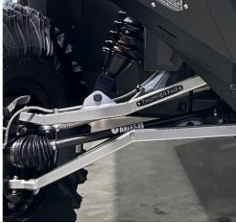
FIG 22 - Mount the brake lines to the upper control arm using zip ties
