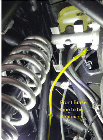
FIG 8 - Replace front brake lines
