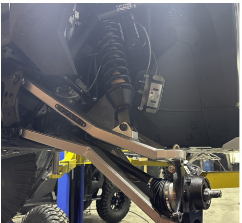
FIG 17 - Mount shock to the upper control arm
