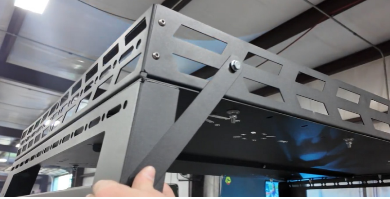
FIG 7 - Fasten the Front gussets from the Lower Side Panels to Upper Basket
