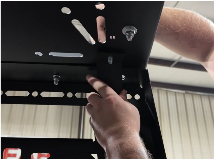
FIG 8 - Mount the Rear Gussets to the Lower Side Panels and Upper Basket
