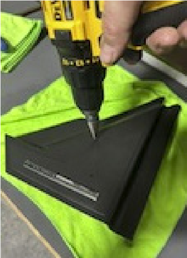
FIG 2 & FIG 3 - Drill holes in A-Pillar Covers
