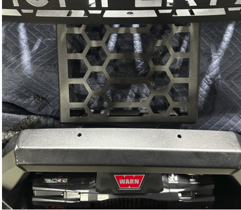
FIG 12 - Drill holes in Thumper Fab Bull Bar using a 3/8" Drill Bit
