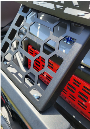
FIG 13 & FIG 14 - Fasten Mount Bracket to Bull Bar using a 13mm socket
