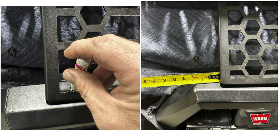
FIG 10 & FIG 11 - Mark Bull Bar to prepare for Drilling
