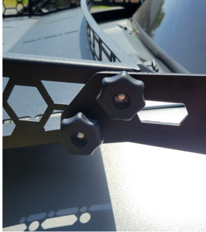
FIG 6 - Fasten Main Basket to Rear Mount Brackets
