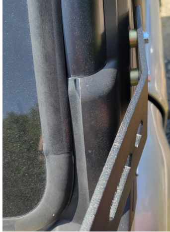
FIG 4 - Fasten Rear Mount Brackets to vehicle using a 13mm socket
