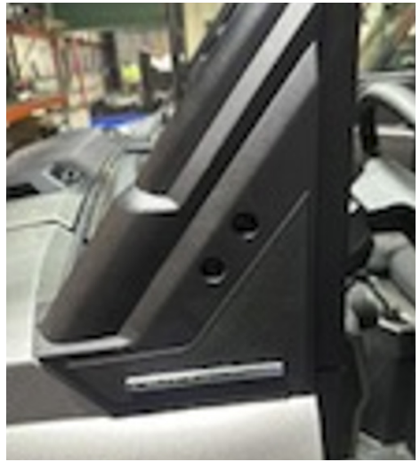
FIG 2 & FIG 3 - Drill holes in A-Pillar Covers
