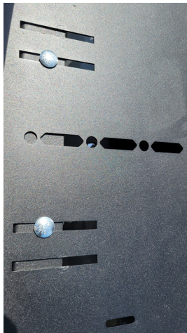
FIG 7 - Fasten front of Main Basket to Bumper Mount
