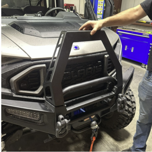
FIG 1 - Fasten Bumper Mount Bracket to bumper using a 13mm socket
