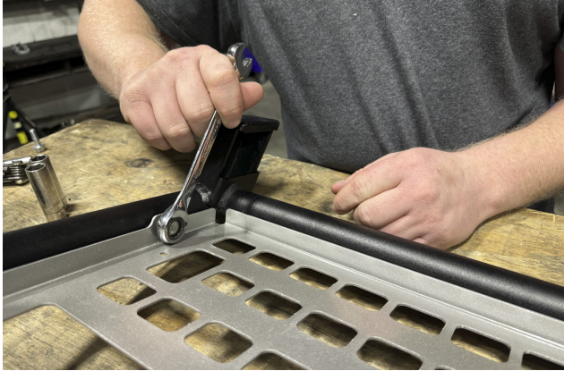
FIG 1 - Fasten Panel (2) to Frame (1) using 13mm Wrench
