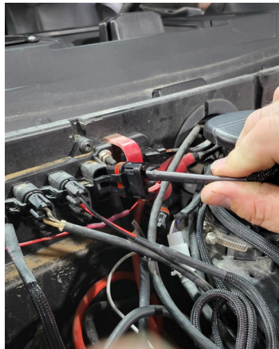
FIG 18 - Plug in Thumper Fab pulse bar pigtail
