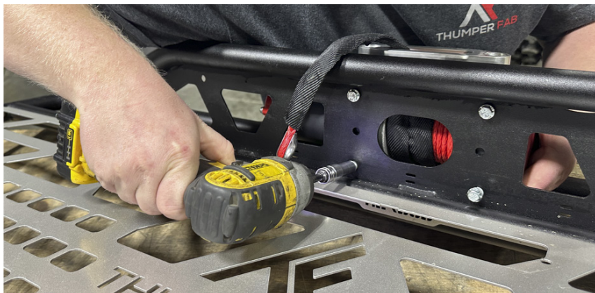
FIG 3 - Fasten Winch (6) to Frame (1) using 10mm Socket
