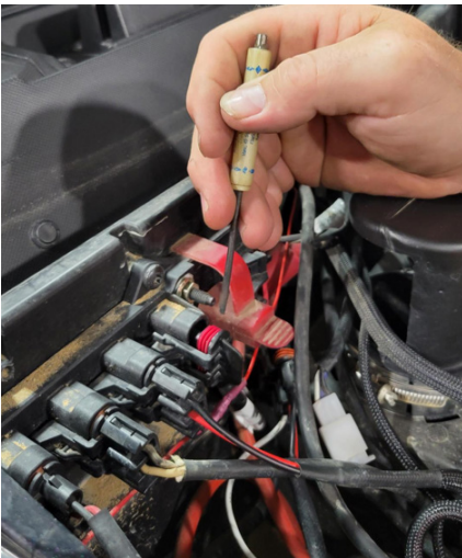
FIG 17 - Remove unused Pulse Bar Plug
