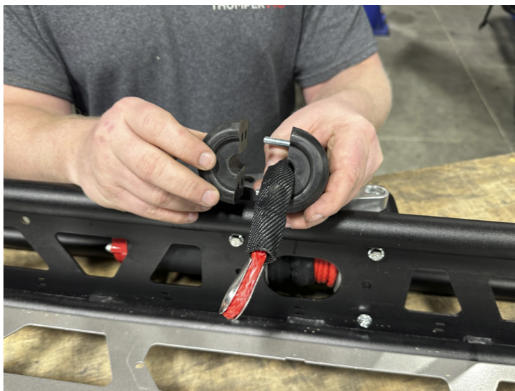
FIG 4 - Fasten Winch Stop (4) to Cable of Winch (6) using a 10mm Socket
