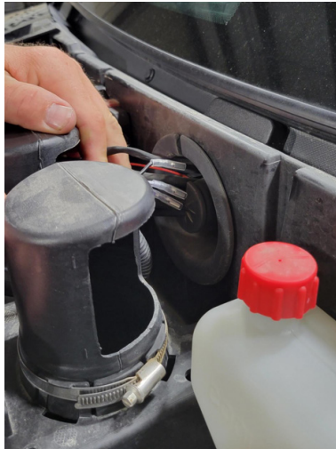
FIG 20 - Feed switch terminals through grommet in firewall
