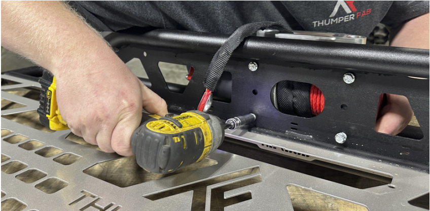
FIG 3 - Fasten Winch (6) to Frame (1) using 10mm Socket
