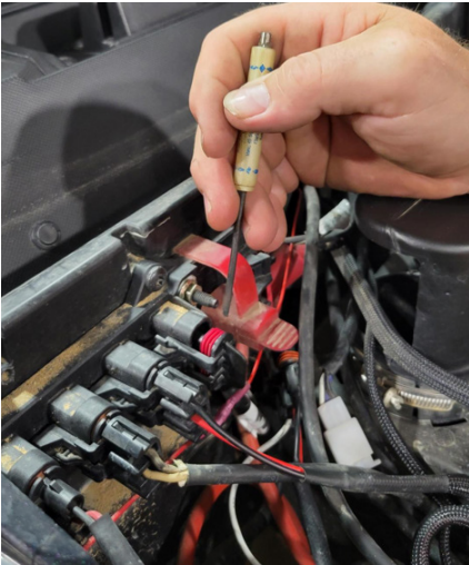
FIG 19 - Remove unused Pulse Bar Plug
