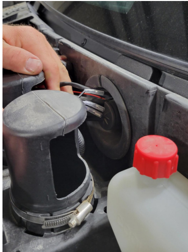
FIG 22 - Feed switch terminals through grommet in firewall
