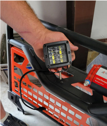
FIG 16 - Fasten Cube Light to Headache Rack
