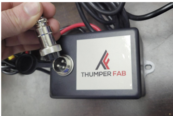
FIG 11 - Plug manual switch harness into winch contactor box
