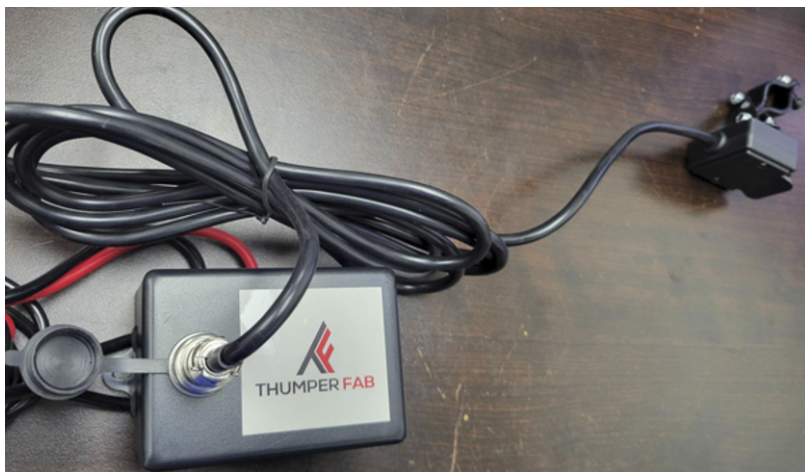
FIG 12 - Tighten switch harness to contactor box
