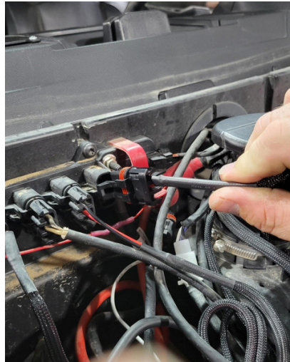
FIG 20 - Plug in Thumper Fab pulse bar pigtail
