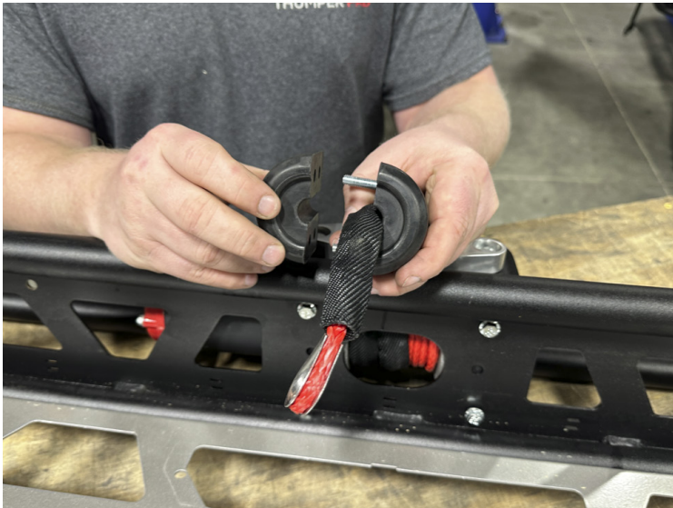
FIG 4 - Fasten Winch Stop (4) to Cable of Winch (6) using a 10mm Socket
