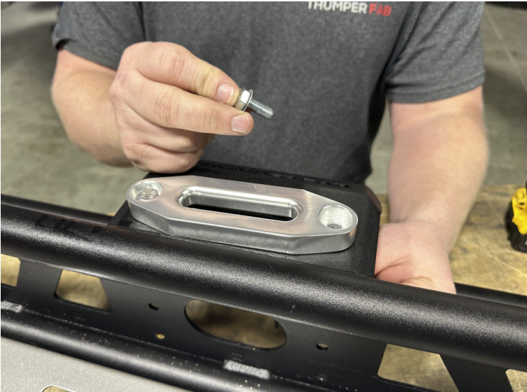
FIG 2 - Fasten Fairlead (5) to Frame (1) using 13mm Socket and 14mm Wrench
