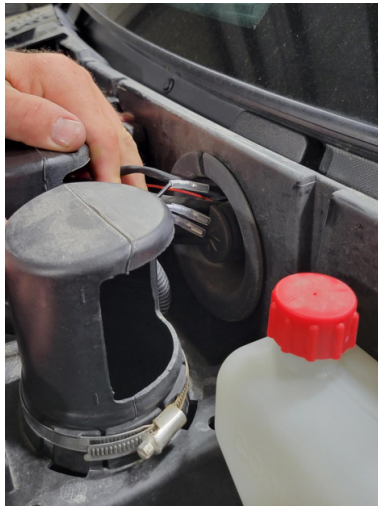
FIG 19 - Feed switch terminals through grommet in firewall
