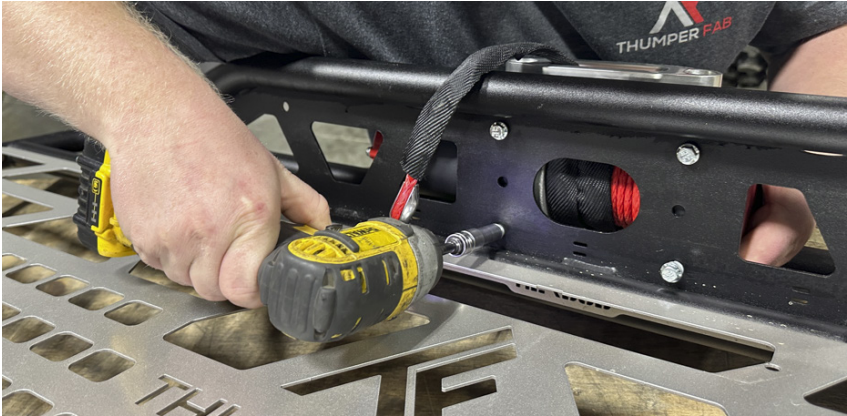
FIG 3 - Fasten Winch (6) to Frame (1) using 10mm Socket
