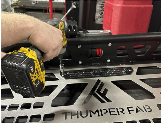
FIG 8 - Fasten Rear Cab Light to Insert Panel (2) using a 5/32" Allen and 7/16" Wrench
