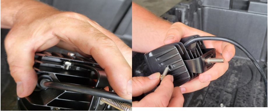
FIG 11 & FIG 12 - Fasten Cube Light to Mount Bracket
