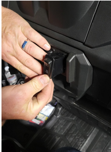
FIG 21 - Snap switch into place in dash
