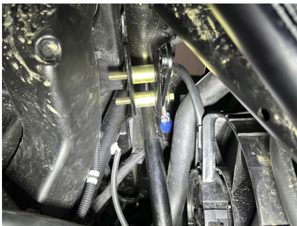
FIG 1 - Mount Front Lift Bracket and Spacers
