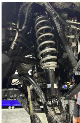
FIG 3 & FIG 4 - Mount Front Shock to Front Lift Brackets
