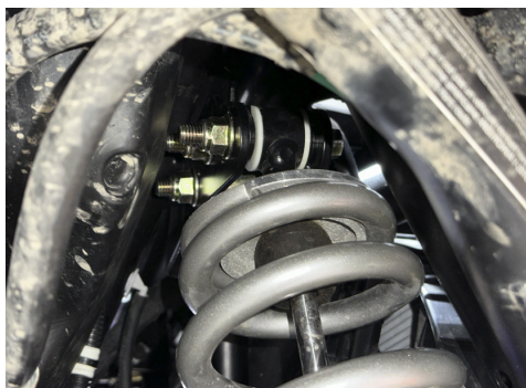
FIG 3 & FIG 4 - Mount Front Shock to Front Lift Brackets
