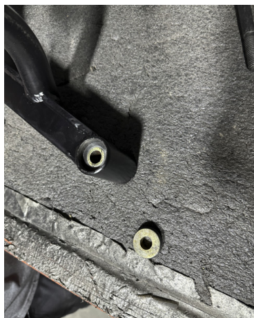
FIG 5 & FIG 6 - Remove and install OEM Bushings into Thumper Fab Control Arms
