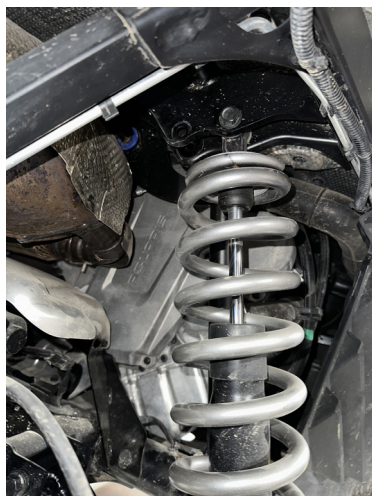
FIG 9 - Mount Rear Shock to the Frame
