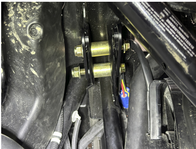
FIG 2 - Mount remaining Front Lift Brackets
