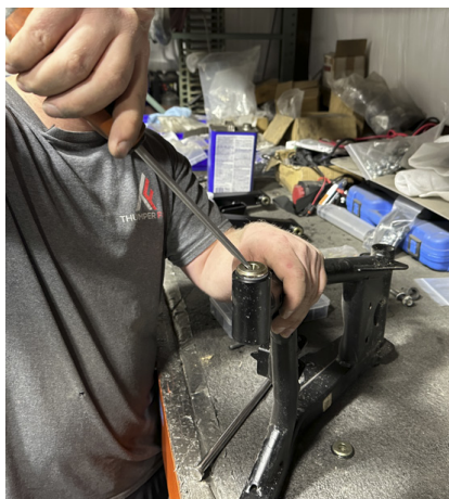
FIG 5 & FIG 6 - Remove and install OEM Bushings into Thumper Fab Control Arms
