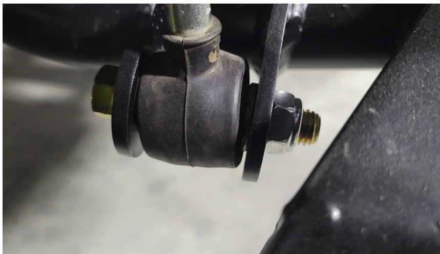
FIG 11 - Mount Sway Bar to Lower Control Arms
