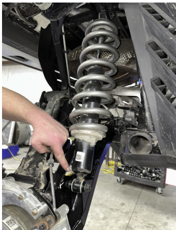
FIG 10 - Mount Rear Shock to Lower Control Arm
