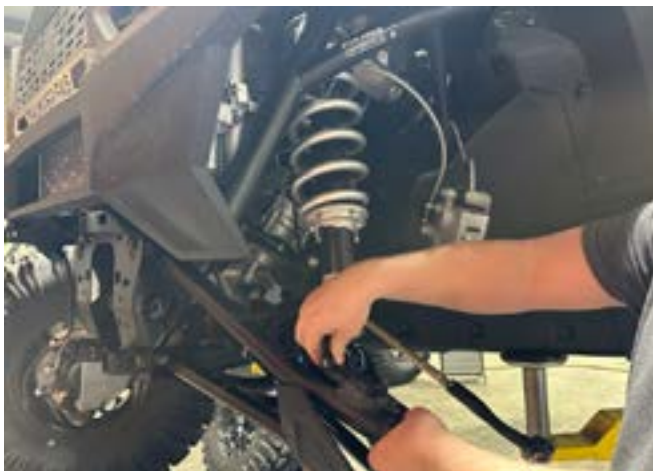
FIG 5 - Disconnect Shock from the Upper Control Arm
