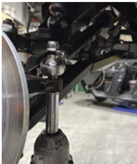
FIG 19 - Mount the Tie Rod to the Hub
