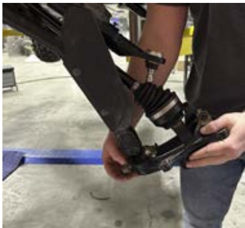
FIG 7 - Disconnect Lower Ball Joint from the Knuckle
