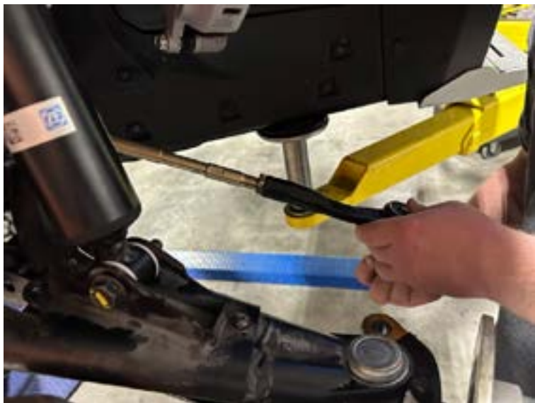
FIG 2 - Disconnect Tie Rod from Knuckle
