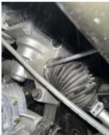
FIG 26 - Remove clamp holding Steering Boot to Steering Rack
