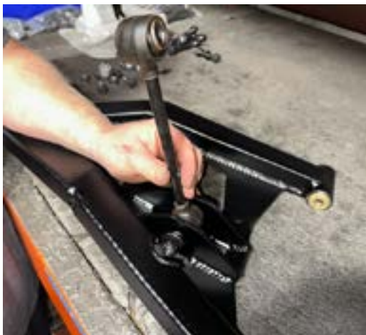
FIG 11 - Remove Upper Control Arm
