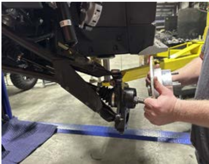
FIG 4 - Remove Hub and Rotor
