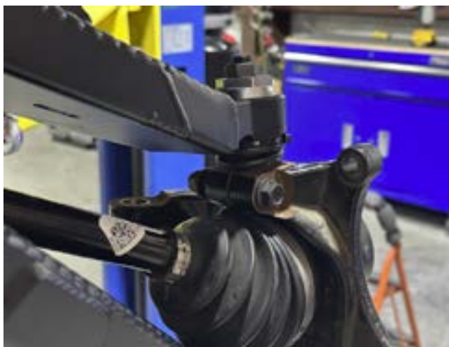
FIG 15 - Fasten the Upper Ball Joint to the Knuckle
