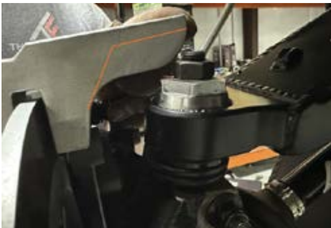
FIG 20 - Mark Rock Gaurd for clearancing (If using TF Elite)
