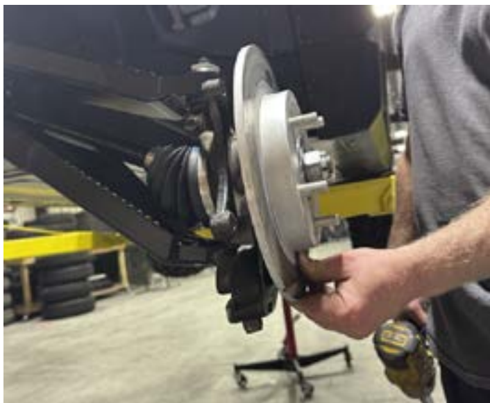
FIG 17 - Slide the Rotor onto the Hub
