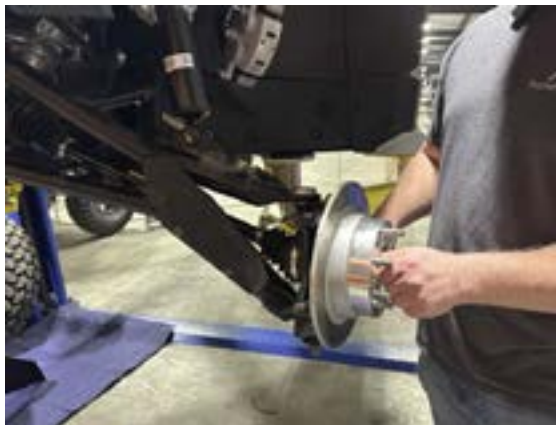
FIG 3 - Remove Axle nut
