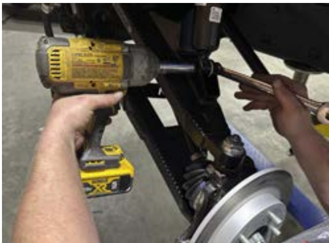
FIG 18 - Mount Shock to Upper Control Arm
