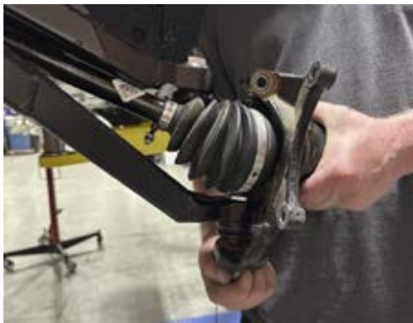
FIG 14 - Mount Lower Ball Joint to Knuckle
