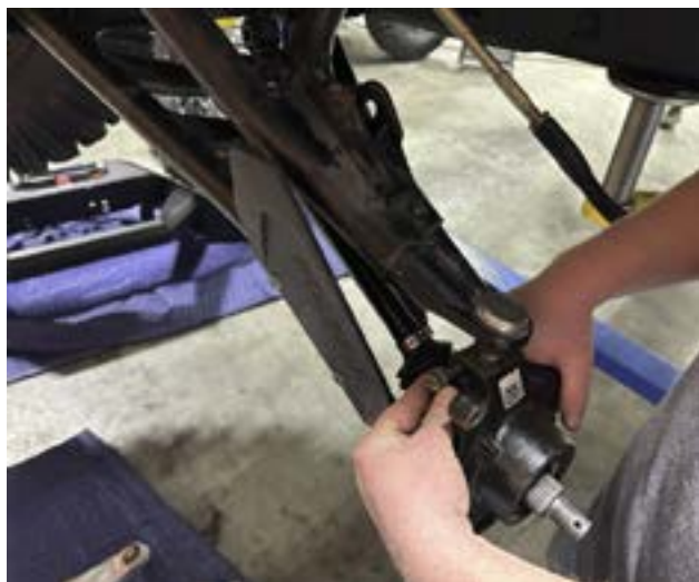
FIG 6 - Disconnect Upper Ball Joint from Knuckle
