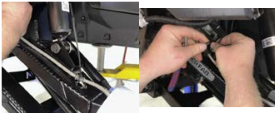
FIG 24 & FIG 25 - Fasten Brake Line to Upper Control Arm
