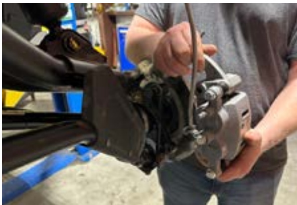
FIG 1 - Disconnect Brake Caliper from Knuckle
