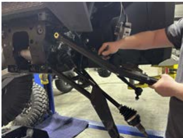
FIG 9 - Remove Upper Control Arm
