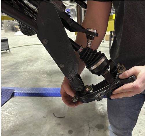
FIG 7 - Disconnect Lower Ball Joint from the Knuckle
