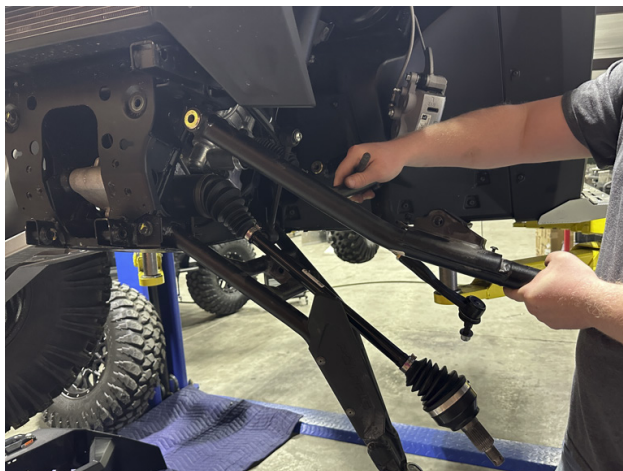
FIG 9 - Remove Upper Control Arm
