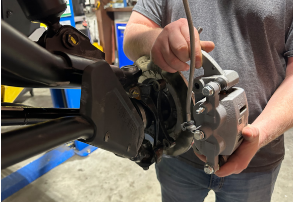
FIG 1 - Disconnect Brake Caliper from Knuckle
