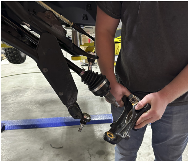
FIG 8 - Remove the Knuckle
