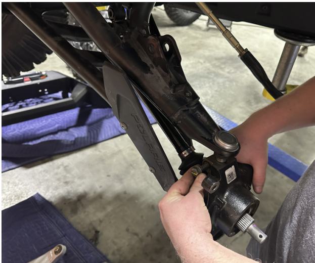
FIG 6 - Disconnect Upper Ball Joint from Knuckle
