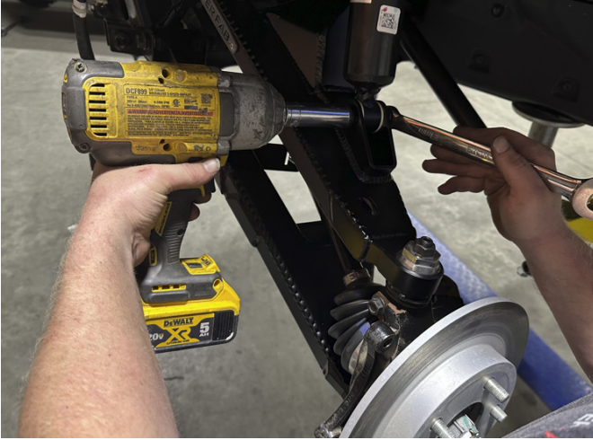
FIG 18 - Mount Shock to Upper Control Arm
