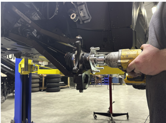
FIG 16 - Mount Hub to Knuckle
