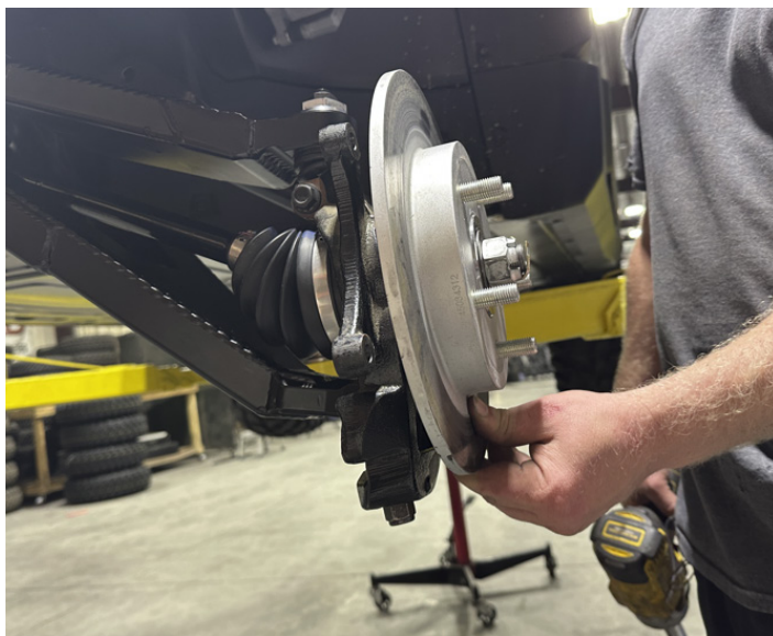
FIG 17 - Slide the Rotor onto the Hub
