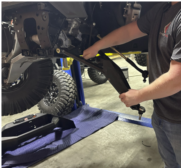
FIG 10 - Remove Lower Control Arm
