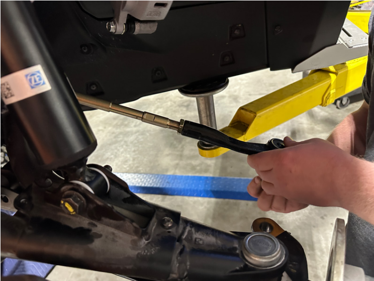
FIG 2 - Disconnect Tie Rod from Knuckle
