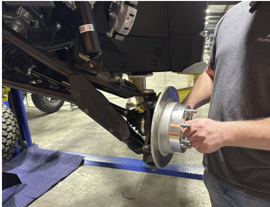
FIG 3 - Remove Axle nut
