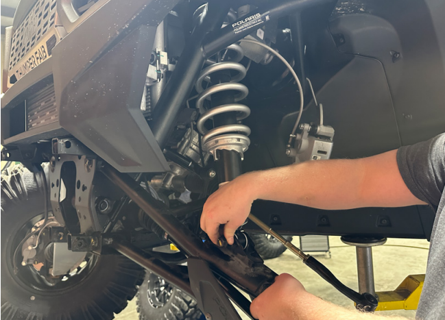
FIG 5 - Disconnect Shock from the Upper Control Arm
