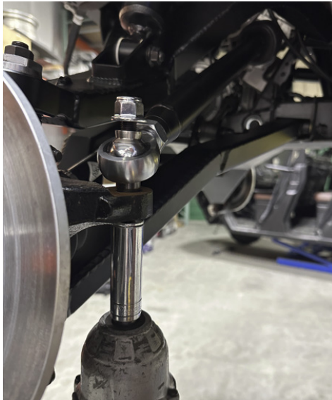
FIG 19 - Mount the Tie Rod to the Hub
