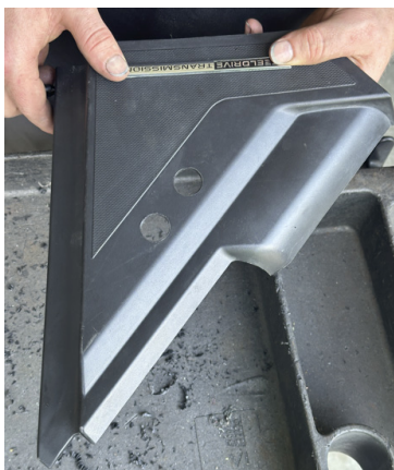
FIG 1 & FIG 2 - Drill out dimples in A Pillar covers
