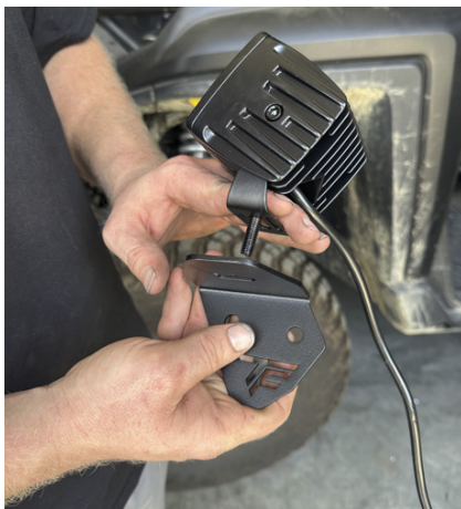
FIG 4 - Mount the Light to the Pod Light Mount Brackets
