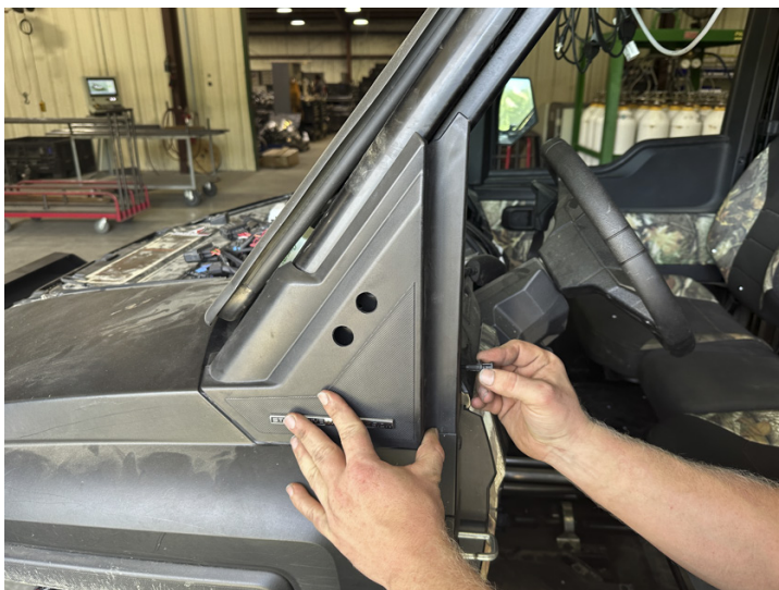
FIG 3 - Resinstall A-Pillar Plastic cover
