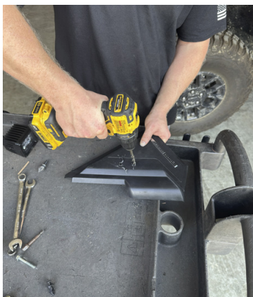
FIG 1 & FIG 2 - Drill out dimples in A Pillar covers
