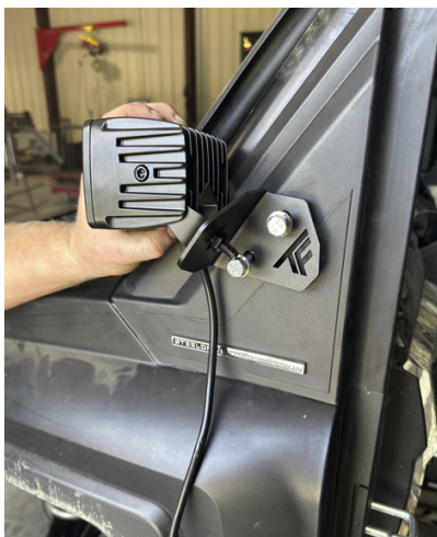
FIG 5 - Fasten the light mount brackets to the vehicle
