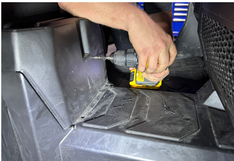
FIG 6 - Drill the marked holes using an 1/8" drill bit
