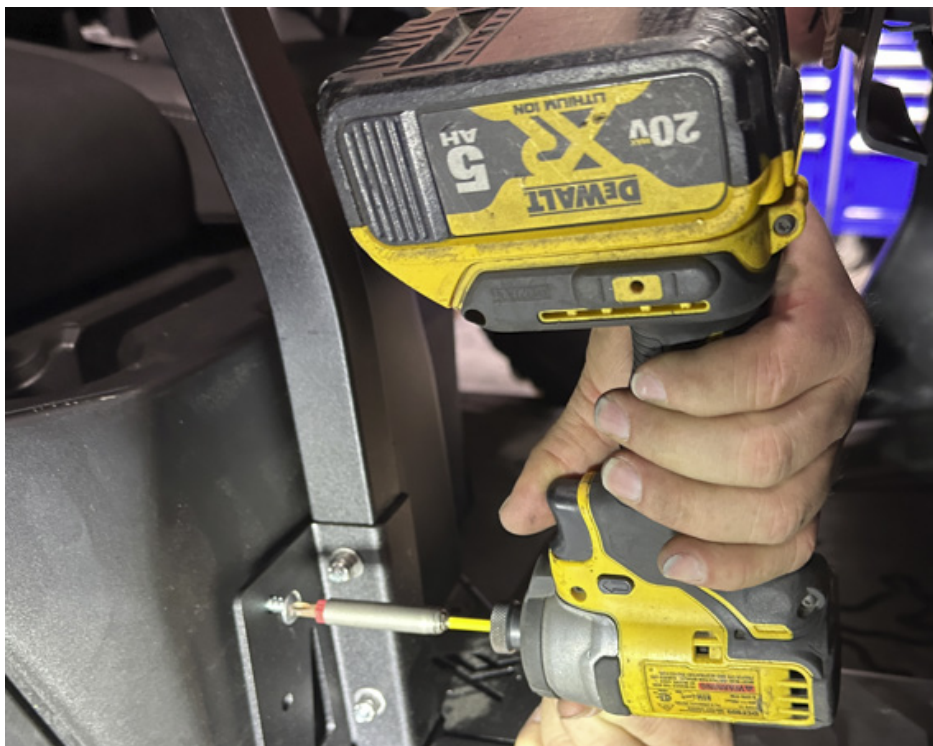
FIG 7 - Mount the Gun Mount Assembly to the Floorboard
