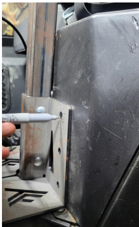
FIG 5 - Mark holes to be drilled using Attachment Plate as a template
