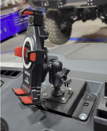
FIG 6 & 7 - Fasten phone charging unit / phone mount to ball mount using the adjustable swivel mount
