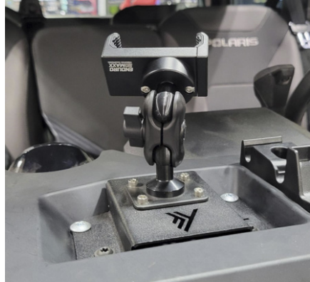
FIG 6 & 7 - Fasten phone charging unit / phone mount to ball mount using the adjustable swivel mount
