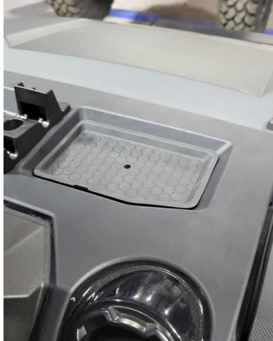
FIG 1 - Remove rubber cover using a flat head screwdriver
