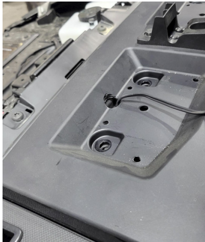
FIG 2 - Drill Hole for wires to run through using 5/8" drill bit
