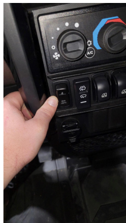
FIG 14 & FIG 15 - Wire Switch and Install in Dash
