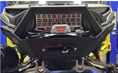
FIG 11 - Primary Winch Mounting Position. Mount Fairlead and Winch, wire according to winch manufacturers instructions
