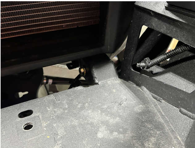
FIG 9 - Loosely Fasten upper mounts using 15mm Socket and 15mm Wrench
