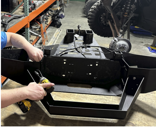
FIG 8 - Fasten Bull Bar (6) and Shims (7) to bumper using 13mm Socket
