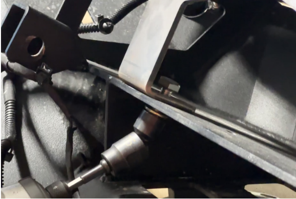
FIG 5 - Loosley fasten lower mount for Small Winch Cover Plate using 15mm Socket and 18mm Wrench
