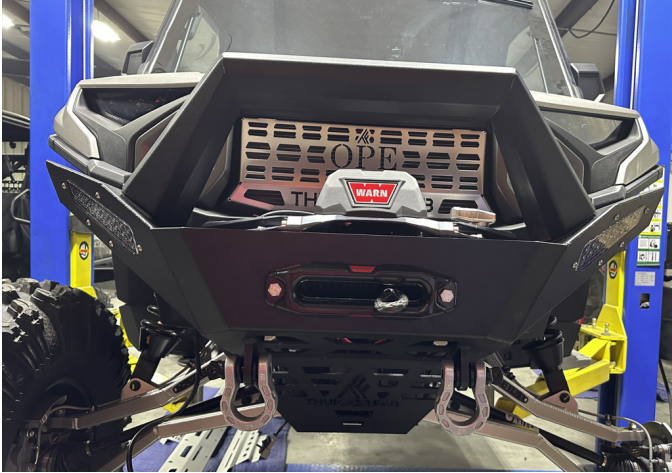
FIG 1 - Front Bumper with Bull Bar Option, OEM Lights Relocated, and Big Winch
