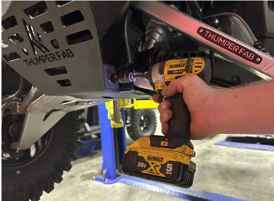
FIG 10 - Fasten Lower bumper mounting hardware using 18mm Socket and 18mm Wrench. Tighten Upper mounting hardware fully afterwards
