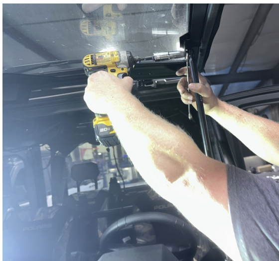
FIG 14 - Disconnect Gas Shocks and remove Windshield
