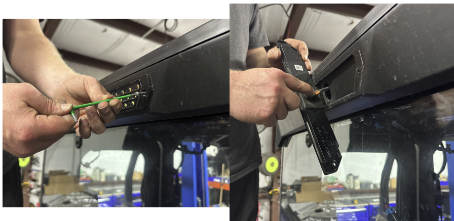
FIG 15 & FIG 16 - Remove Bed light from the Roof
