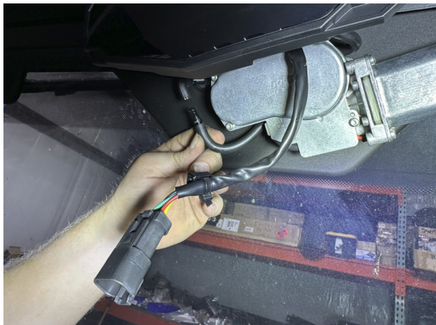
FIG 13 - Disconnect Wiper Motor and Wiper Fluid line
