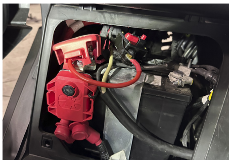
FIG 40 & FIG 41 - Connect Power Wire to Breaker and Breaker and ground wire to Battery
