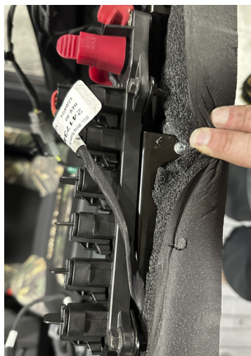
FIG 19 & FIG 20 - Mount Rear Pulse Bar to Roll Cage
