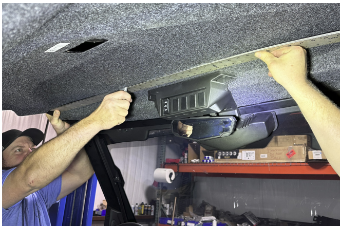
FIG 38 - Tighten Roof, Install and Trim Front Headliner
