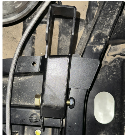
FIG 5 & FIG 6 - Mount Relocation Bracket into Position
