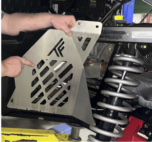
FIG 1 - Remove Inner Fender Liner
