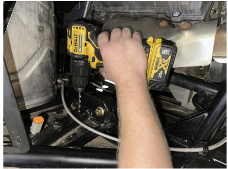
FIG 7 & FIG 8 - Drill hole in frame using Bracket as a template
