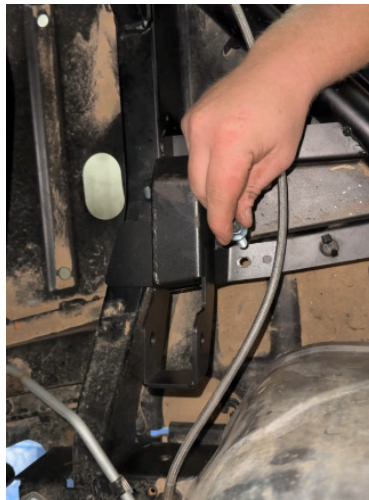
FIG 9 - Mount the Relocation Bracket to the Frame
