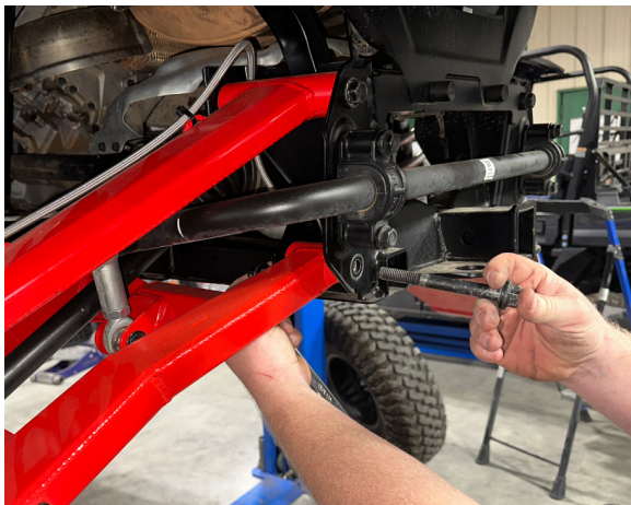
FIG 1 - Remove OEM Lower Control Arm Mounting Bolts
