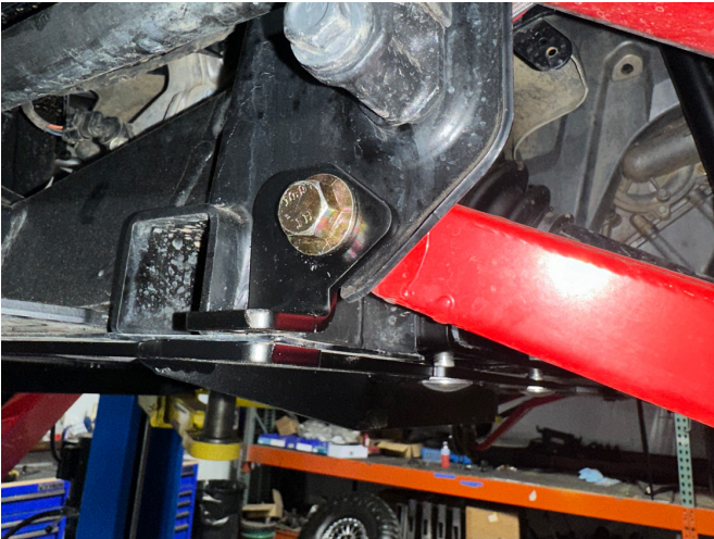
FIG 4 - Loosley Mount Rear Braces to Vehicle
