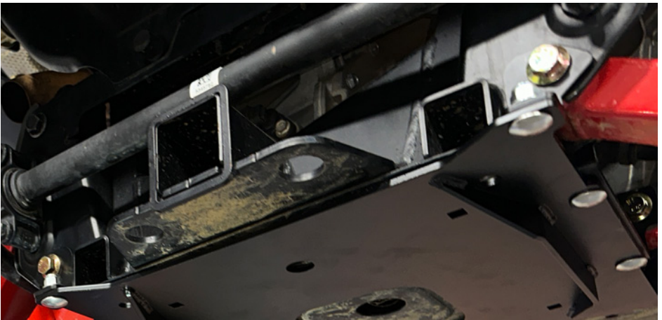
FIG 6 - Install remaining Carriage Bolts
