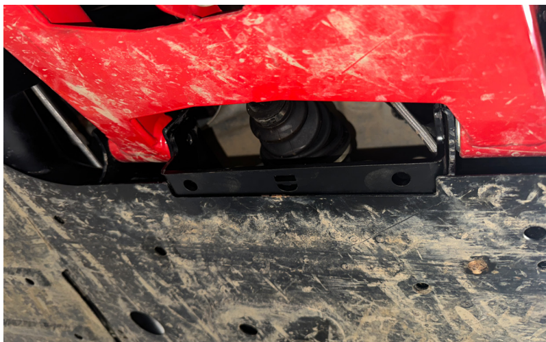
FIG 2 - Insert Middle Braces into place
