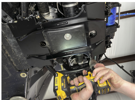
FIG 4 & FIG 5 - Drill holes through frame using the Base as a template
