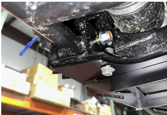
FIG 6 - Loosley mount Forward Rear Brackets Driver & Passenger to Frame
