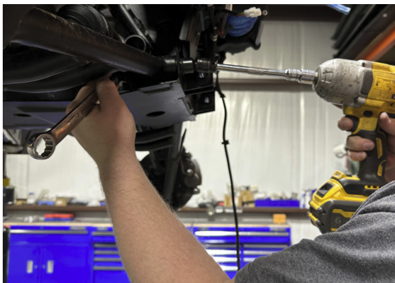
FIG 1 - Remove the Lower Control Arm Mounting Bolts
