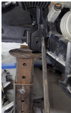
FIG 2 & FIG 3 - Loosley mount Base to Vehicle Frame
