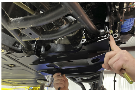
FIG 2 & FIG 3 - Loosley mount Base to Vehicle Frame
