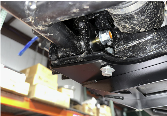
FIG 5 - Loosley mount Forward Rear Brackets Driver & Passenger to Frame
