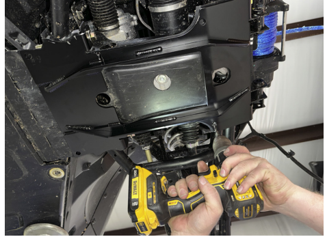
FIG 3 & FIG 4 - Drill holes through frame using the Base as a template
