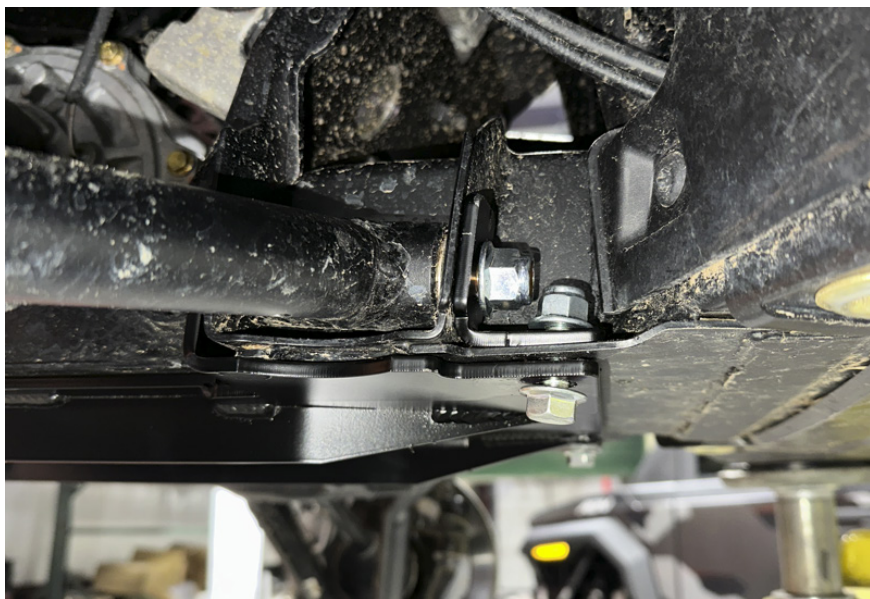
FIG 6 - Mount AFT Rear Brackets Driver & Passenger
