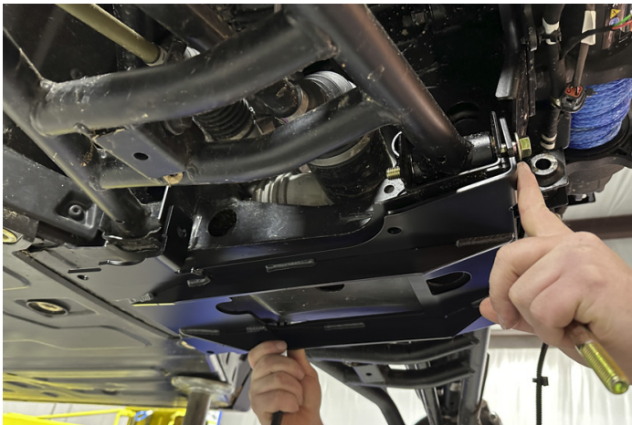
FIG 2 - Loosely mount Base to Vehicle Frame
